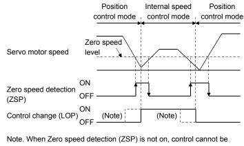
changed if Control change (LOP) is switched on-off. If Zero speed detection (ZSP) switches on after that, control cannot be changed.
