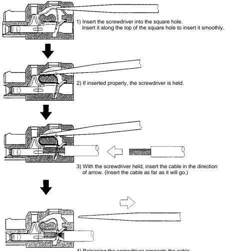
4) Releasing the screwdriver connects the cable.
