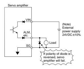
Note. If the voltage drop (maximum of 2.6V) interferes with the relay operation, apply high voltage (up to 26.4V) from external source.
