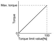
A relationship between the applied voltage of the analog torque limit (TLA) and the torque limit value of the servo motor is shown below. Torque limit values will vary about 5% relative to the voltage depending on products.
