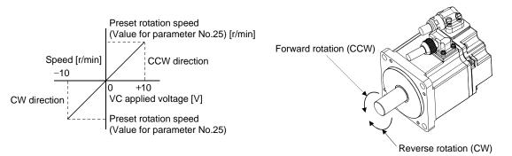
The following table indicates the rotation direction according to forward rotation start (ST1) and reverse rotation start (ST2) combination.
