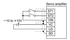
2) Speed selection 1 (SP1), speed selection 2 (SP2), speed selection 3 (SP3) and speed command value by making speed selection 1 (SP1), speed selection 2 (SP2) and speed selection 3 (SP3) usable by setting of parameter No.43 to 47, you can choose the speed command values of internal speed commands 1 to 7.
