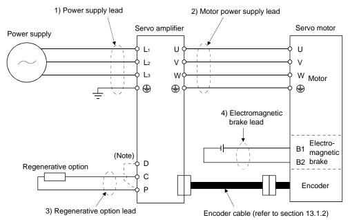
Note. When using the regenerative option, always remove the wiring across D-P.
