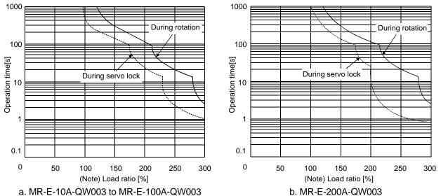
Note. If operation that generates torque more than 100% of the rating is performed with an abnormally high frequency in a servo motor stop status (servo lock status) or in a 30r/min or less low-speed operation status, the servo amplifier may fail even when the electronic thermal relay protection is not activated.
