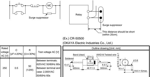
Note that a diode should be installed to a DC relay, DC valve or the like.
