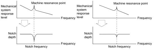
When machine resonance is large and frequency is low When machine resonance is small and frequency is high
