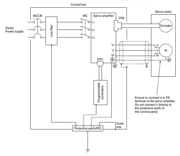
Note. For 1-phase 230VAC, connect the power supply to L<sub>1</sub>, L<sub>2</sub> and leave L<sub>3</sub> open. Refer to section 1.3 for the power supply specification.
