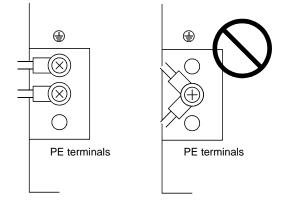
(c) If an earth leakage circuit breaker is used, always earth the protective earth (PE) terminal of the servo amplifier to prevent an electric shock.
