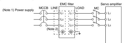
Note 1. For 1-phase 230VAC power supply, connect the power supply to  $L_{1}$ , $L_{2}$  and leave  $L_{3}$  open. 2. Connect when the power supply has earth.
