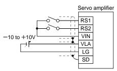
Speed selection 1(SP1)/speed selection 2(SP2)/speed selection 3(SP3) and speed limit values Choose any of the speed settings made by the internal speed limits 1 to 7 using speed selection 1(SP1), speed selection 2(SP2) and speed selection 3(SP3) or the speed setting made by the analog speed limit (VLA), as indicated below.
