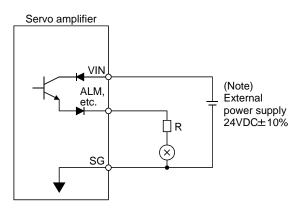
Note. If the voltage drop (maximum of 2.6V) interferes with the relay operation, apply high voltage (up to 26.4V) from external source.
