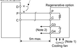
Note 1. When using the MR-RB50, forcibly cool it with a cooling fan  $(92 \times 92, \text{ minimum air flow: } 1.0\text{m}^3)$ .
