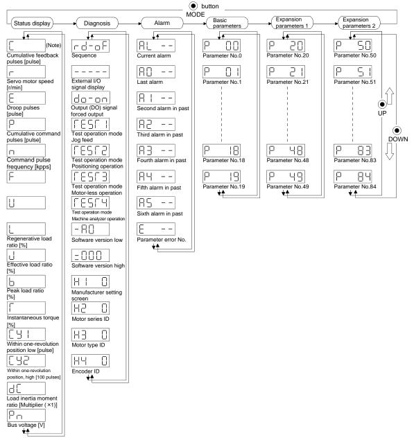
Note. The initial status display at power-on depends on the control mode.
