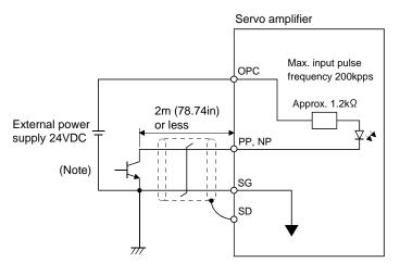
Note. Pulse train input interface is comprised of a photo coupler.
