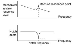
You can use the machine resonance suppression filter 1 (parameter No.58) and machine resonance suppression filter 2 (parameter No.59) to suppress the vibration of two resonance frequencies. Note that if adaptive vibration suppression control is made valid, the machine resonance suppression filter 1 (parameter No.58) is made invalid.
