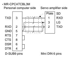
When fabricating the cable, refer to the connection diagram in this section. Though this connection diagram is not the connection diagram of the QC30R2, it is identical in functions.
