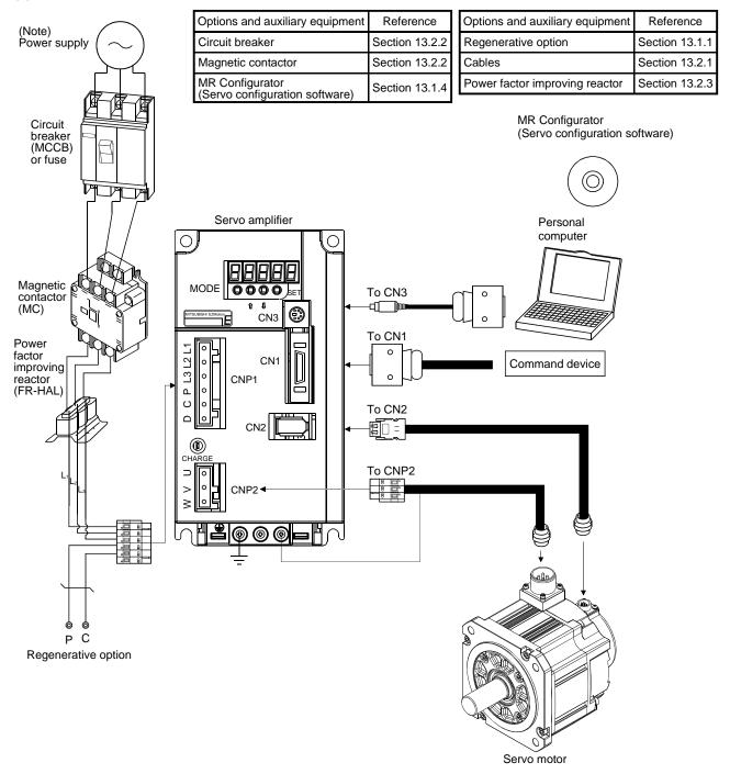
Note. Refer to section 1.3 for the power supply specification.
