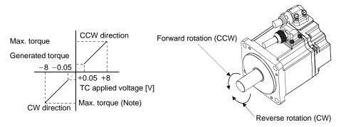
Generated torque limit values will vary about 5% relative to the voltage depending on products. Also the torque may vary if the voltage is low (-0.05 to +0.05V) and the actual speed is close to the limit value. In such a case, increase the speed limit value.
