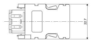
(3) CN3 Connector (Marushin electric mfg) Connector: MP371/6
