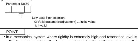
difficult to occur, setting the low-pass filter to be "invalid" may increase the servo system response level to shorten the settling time.
