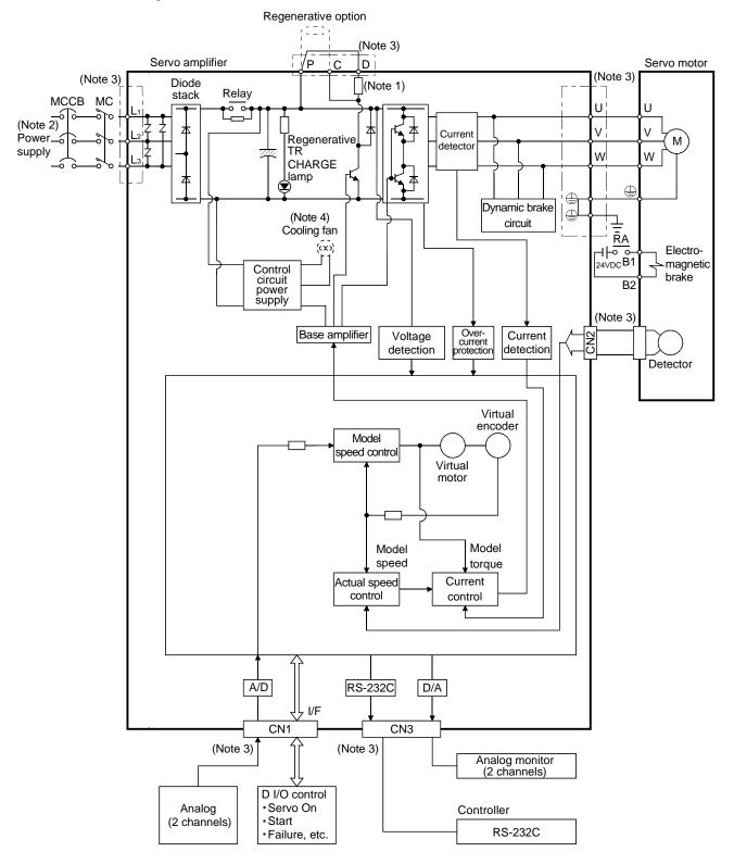
Note 1. The built-in regenerative resistor is not provided for the MR-E-10AG-QW003/MR-E-20AG-QW003.
