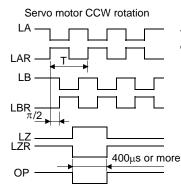
Time cycle (T) is determined by the settings of parameter No.27 and 54.
