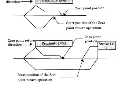
Note) When returning to the Zero point from a position that exceeds the dog, if the dog cannot be detected, the axis will stop at the maximum limit switch in the direction opposite the Zero point return direction.
