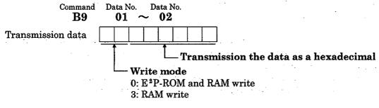
When the general-purpose register (Rx) value is changed frequently through communication, set this value to "3" and change only the data on RAM. Frequent changing of the E<sup>2</sup>P-ROM value will result in an E<sup>2</sup>P-ROM fault due to excess of the E<sup>2</sup>P-ROM write times.
