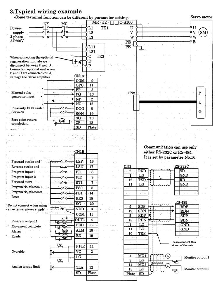
Note) Input / output function signals can be changed by the Setup-S/W.
