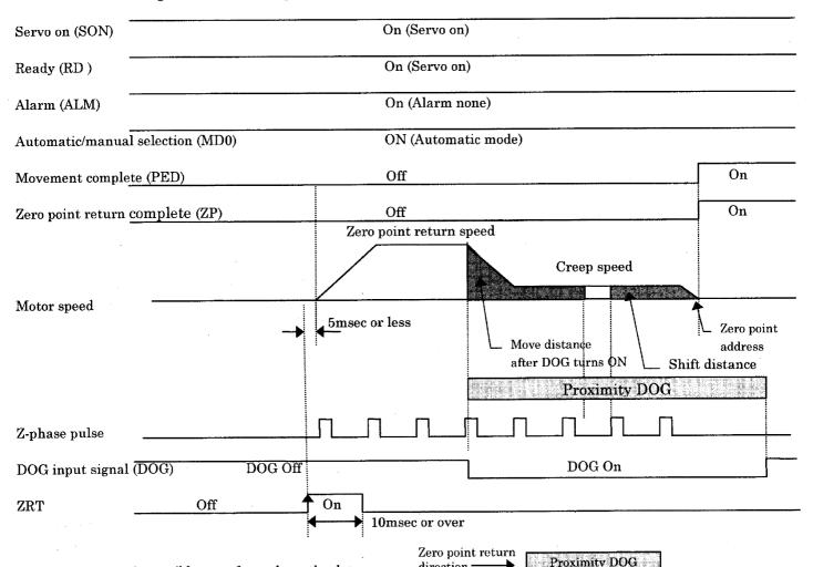
Zero point return is possible even from above the dog. The axis will move in the reverse direction from the Zero point return direction, and then will return to and decelerate to a stop at the front end of the dog. After that, the normal Zero point return will be carried out automatically.
