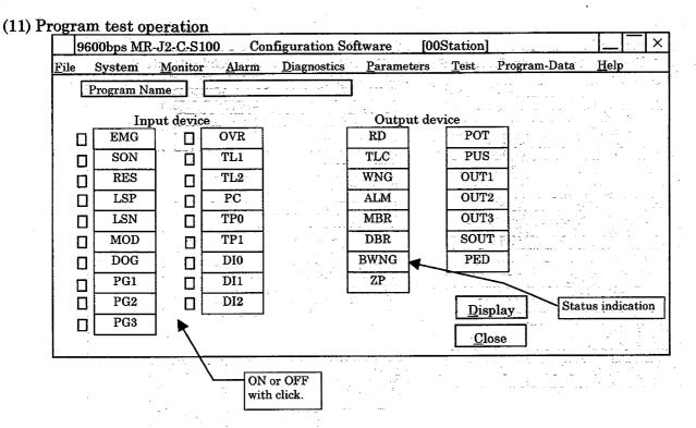
(12) Program test operation [00Station] 9600bps MR-J2-C-S100 Configuration Software  $\underline{\mathrm{T}}\mathrm{est}$ Program-Data <u>H</u>elp Parameters Diagnostics System Monitor <u>A</u>larm Program Program display (The executing step is indicated with turn-over) Close
