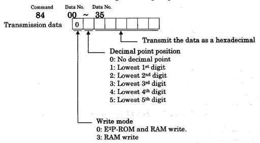
If the parameters are changed many times with the communication, it must be set "3" and changing the parameters to only RAM data. Otherwise, E<sup>2</sup>P-ROM error occurrence.
