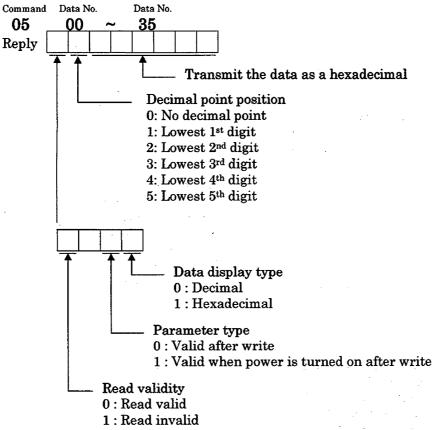
Note) The validity information will change according to the setting of the parameter 19(BLK) parameter write prohibit setting(reference range). If reading is invalidated, the parameter data section will be ignored, and will be processed as if it was not readable.
