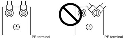
(c) If an earth leakage circuit breaker is used, always earth the protective earth (PE) terminal of the servo amplifier to prevent an electric shock.
