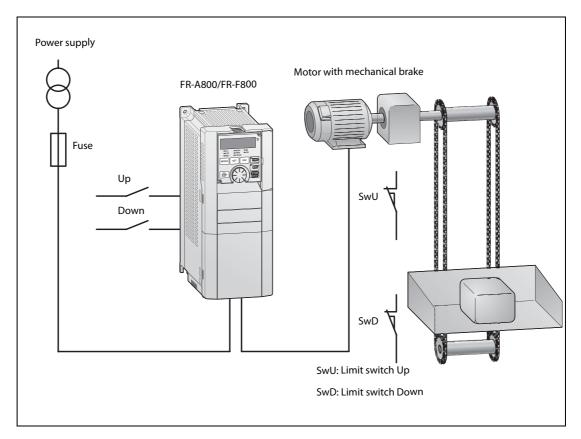
In the wiring diagram on the next page the mechanical brake is controlled via the RUN terminal. The frequency at which the brake is released can be set with parameter 13.
