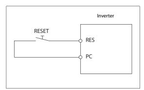
This example shows how to wire the RES terminal for positive logic.
