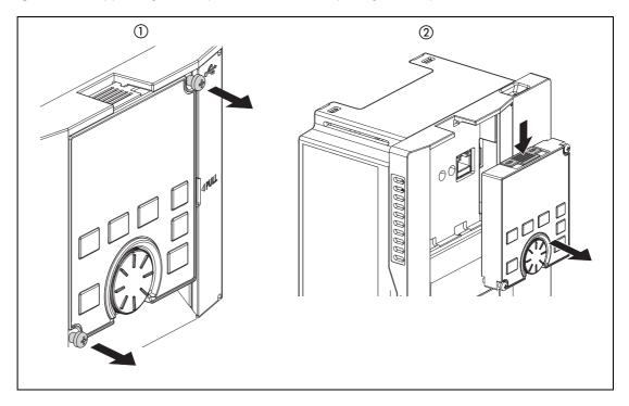
To reinstall the parameter unit, align its connector on the back with the PU connector of the inverter, and insert the parameter unit. After confirming that the parameter unit is fit securely, tighten the screws. (Tightening torque: 0.40 to 0.45 Nm)
