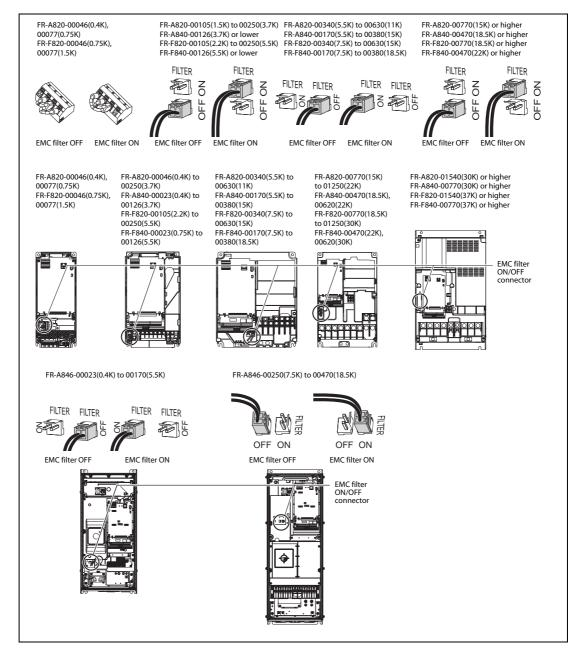
The connector must always be installed, either in the ON position or in the OFF position.
