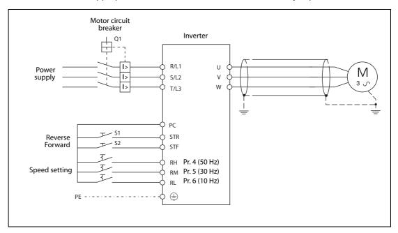
Some external components like pushbuttons and switches are required for this method but it has advantages over performing the test with the parameter unit:
