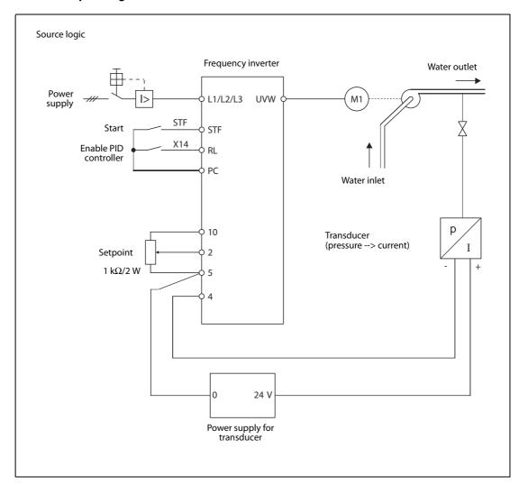
For the PID controller application using the configuration shown above you must also set the inverter parameters shown in the table below, in addition to the basic parameters.
