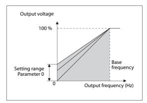
You can use parameter 0 to achieve better performance for starting the motor under load. The base frequency is set in parameter 3.
