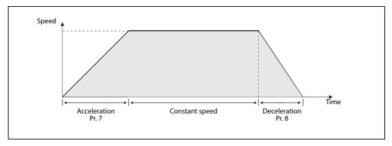
In this example we are going to use an FR-A800 or FR-F800 series inverter to power and control the belt using the speed/time pattern shown in the graph above.
