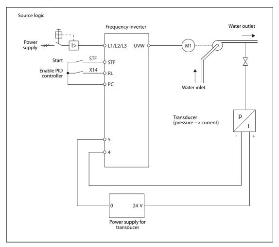
In addition to the basic parameters you must also set the following parameters for this configuration:
