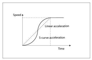
If the material on the belt still shifts when stopping and starting even with a gentle acceleration curve you can solve the problem by programming an S-curve for acceleration and deceleration, as shown in the graph on the left.
