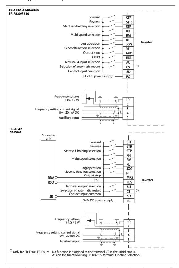
The manuals of the individual frequency inverters also include diagrams showing the connections for controlling the inverter inputs with PLC outputs and with source logic.
