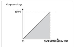
The speed of the connected motor can be adjusted continuously by changing the output voltage and frequency of the inverter.
