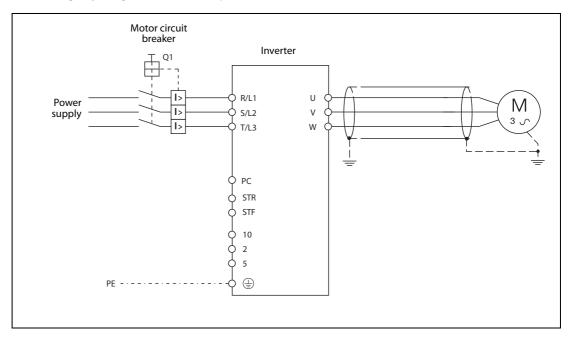
Please note that when the inverter is switched on for the first time control via external signals is activated by default. Press the PU/EXT key of the parameter unit FR-DU08 (HAND/AUTO key for FR-DU08-01) to select the PU operation mode (see section 5.2).
