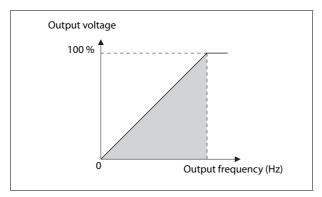
Parameter 3 defines the ratio between the output voltage and the output frequency (V/f pattern).
