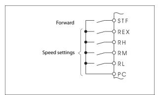
Example for connection of the inverter's RH, RM, RL and REX terminals (in source logic).
