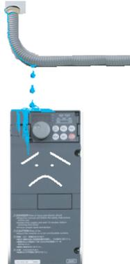
Failure example 2: Inverter failure due to foreign object
