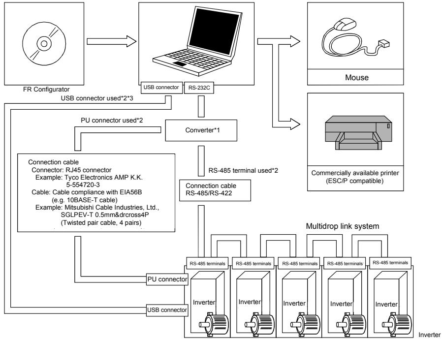
\*1: A commercially available converter is required when the personal computer uses the RS-232C port.
