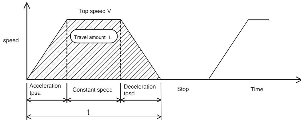
When the top speed is  $V$  [mm/s], travel time is  $t$  [s], acceleration and deceleration times are respectively  $tpsa$  [s] and  $tpsd$  [s], travel amount is  $L$  [mm], and  $tpsa=tpsd$ , their relation is as shown in the following formula.
