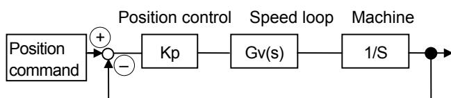
The speed control is assumed as  $G_v(s) = 1$  since the response to the position control is sufficiently high.
