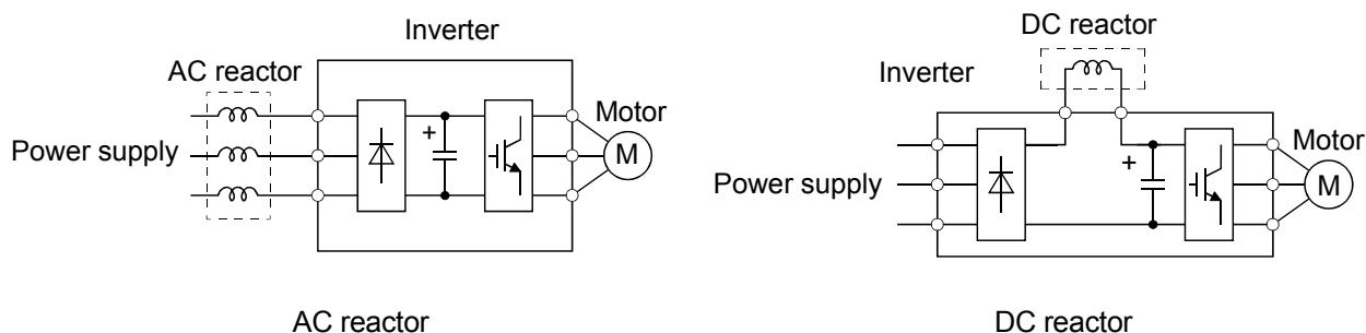
Even for consumers to whom the guideline is not applied, it is recommended to connect a power factor improving reactor in the same manner to avoid possible troubles due to the harmonic current.
