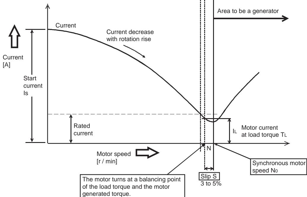
Fig. 1.6 Relationship of motor speed and current
