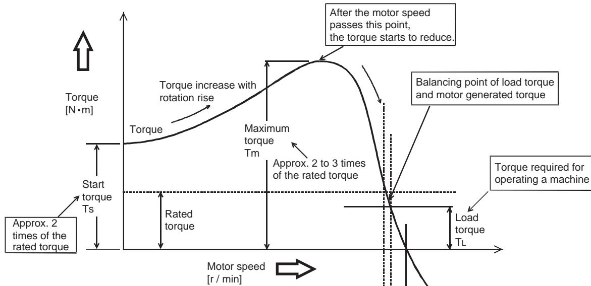
Fig. 1.5 Relationship of motor speed and torque
