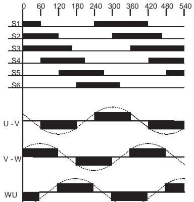
Fig. 2.18 Method to create 3-phase AC
