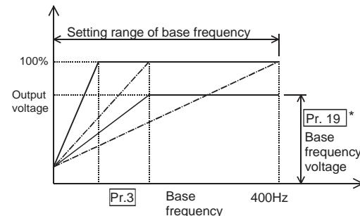
\* If Pr.19 is set to 9999 (factory default), the maximum output voltage will be the same as the power supply voltage.
