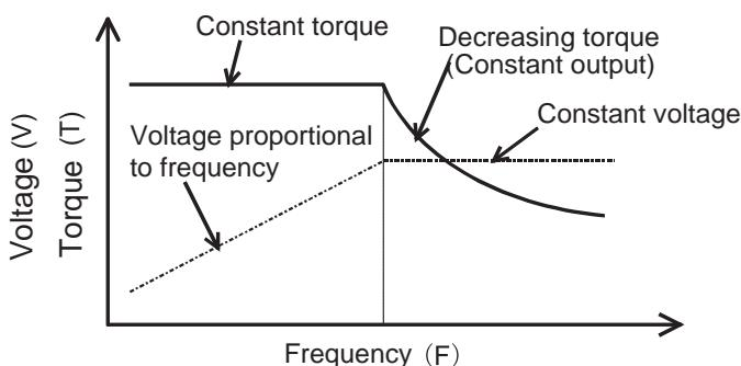
Fig. 2.19 V/F pattern and motor output torque
