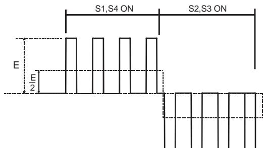
Figure 2.15 Voltage waveform of  $E/2$
