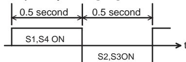
Figure 2.13 1Hz AC waveform
