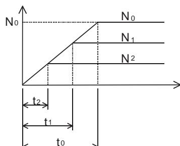
t<sub>0</sub>: Acceleration time up to the reference speed = Acceleration time constant
