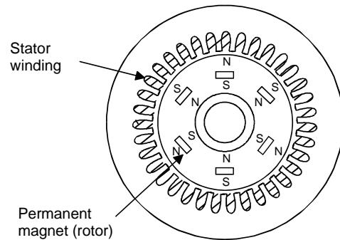
Fig. 1.4 Cross section of PM motor
