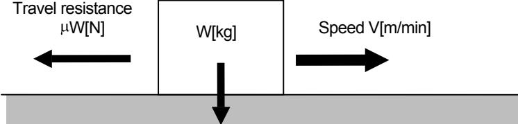
$$P = \frac{\mu WV}{6120\eta} \text{ [kW]} \dots\dots \text{(Formula 4.1)}$$
