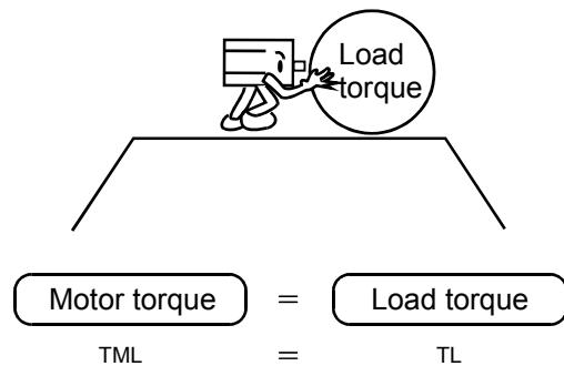
3) Torque required for decelerating to the stop
