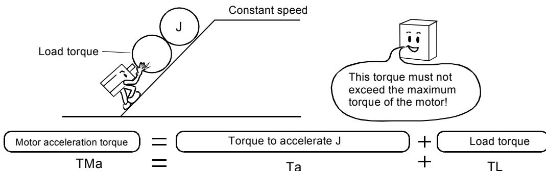
2) Torque required for keeping the load moving at a constant speed
