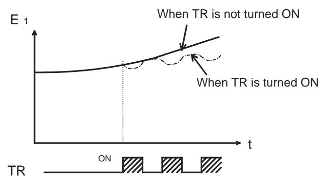
Fig. 2.21 DC voltage (between P and N)
