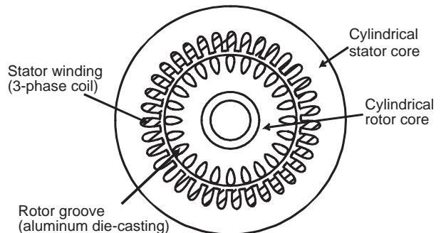
Fig. 1.3 Cross section of 3-phase motor (induction type)
