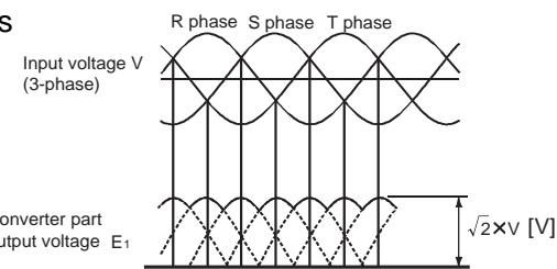
Fig. 2.7 Converter part waveform
