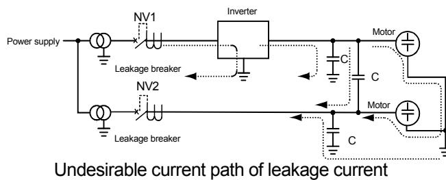
Undesirable current path of leakage current
