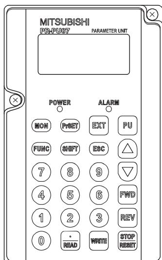
Parameter settings are performed by the operation of the parameter unit (PU) at an operation stop.
