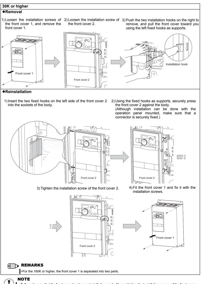
Fully make sure that the front cover has been reinstalled securely. Always tighten the installation screws of the front cover. The same serial number is printed on the capacity plate of the front cover and the rating plate of the converter. Before reinstalling the front cover, check the serial numbers to ensure that the cover removed is reinstalled to the converter from where it was removed.
