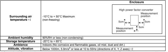
\*1 Surrounding Air Temperature is a temperature measured at a measurement position in an enclosure. Ambient Temperature is a temperature outside an enclosure. \*2 2.9m/s<sup>2</sup> or less for the 160K or higher
