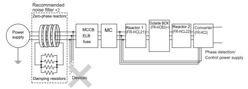
\*4 Line noise filters (FR-BLF, or non-Mitsubishi Electric product RC5128 or FINEMET<sup>®</sup> FT-3KM F/ FT-3KL F series) The RC5128 reactor core is manufactured by Soshin Electric Co., Ltd. and available on the market. FINEMET<sup>®</sup> FT-3KM F/ FT-3KL F series common mode choke core is manufactured by Hitachi Metals, Ltd. and available on the market.
