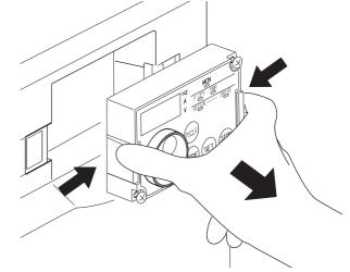
When reinstalling the operation panel, insert it straight to reinstall securely and tighten the screws of the operation panel.
