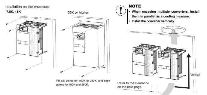
• The converter consists of precision mechanical and electronic parts. Never install or handle it in any of the following conditions as doing so could cause an operation fault or failure.
