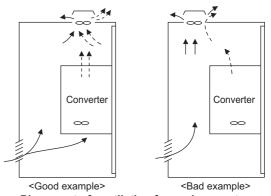
Placement of ventilation fan and converter
