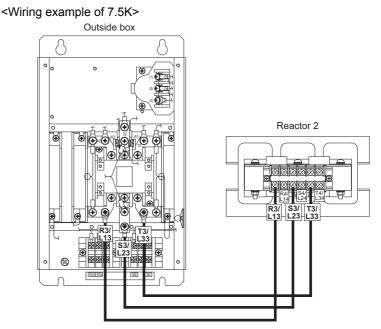
The terminal arrangement differs by capacity. Check the terminal arrangement on 6.3 Outline dimensions (refer to page 154).
