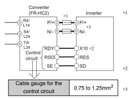
Installation of a fuse is recommended to avoid the damage to spread in case of an inverter failure. Select a fuse according to the motor capacity. When using a motor, of which the capacity is smaller than the inverter capacity by two ranks or more, select the fuse with the capacity that is one rank lower than the inverter capacity. Refer to the fuse selection table on *page 15, 17.*
