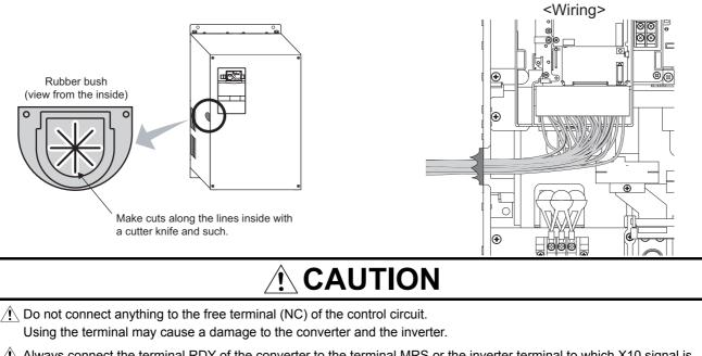
Always connect the terminal RDY of the converter to the terminal MRS or the inverter terminal to which X10 signal is assigned. Also, always connect the terminal SE of the converter to the terminal SD of the inverter. If these are not connected, the converter may be damaged.
