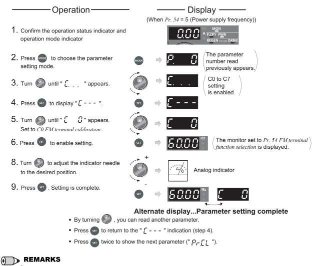
· Calibration can be performed during operation.
