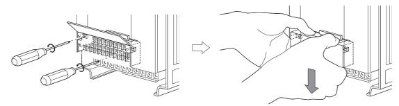
(2) Change the jumper connector set to the sink logic (SINK) on the rear panel of the control circuit terminal block to the source logic (SOURCE).
