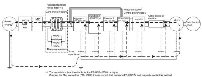
\*2 Suppression effectiveness of the recommended noise filter installed anywhere between the power supply and the reactor 1 (FR-HCL21) remains the same.
