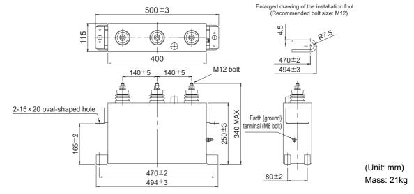
•Filter capacitor alarm detector (MDA-1) (FR-HCC2-H400K, H560K)
