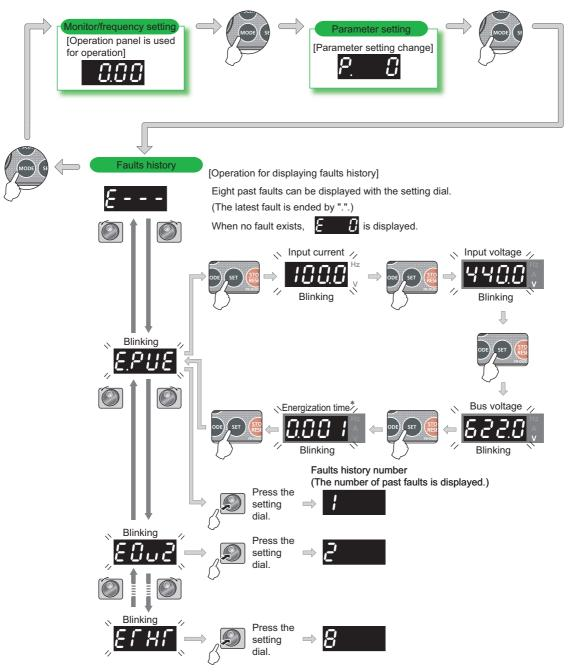
\* The cumulative energization time is accumulated from 0 to 65535 hours, then cleared, and accumulated again from 0. When using the operation panel (FR-DU07-CNV), the time is displayed up to 65.53 (65530h) by regarding 1h = 0.001, and thereafter, it is added up from 0.
