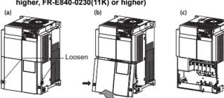
(a) Loosen the screws on the lower front cover. (These screws cannot be removed.)
