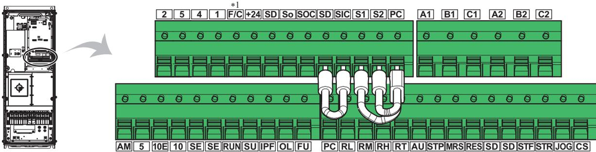
\*1 This terminal operates as terminal FM for the FM type, and as terminal CA for the CA type.
