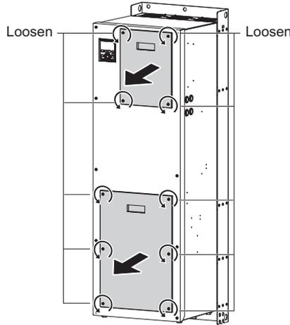
◆ **Installation of the front cover for control circuit inspection and the front cover for main circuit inspection (FR-A846-01800(55K) or higher)**
