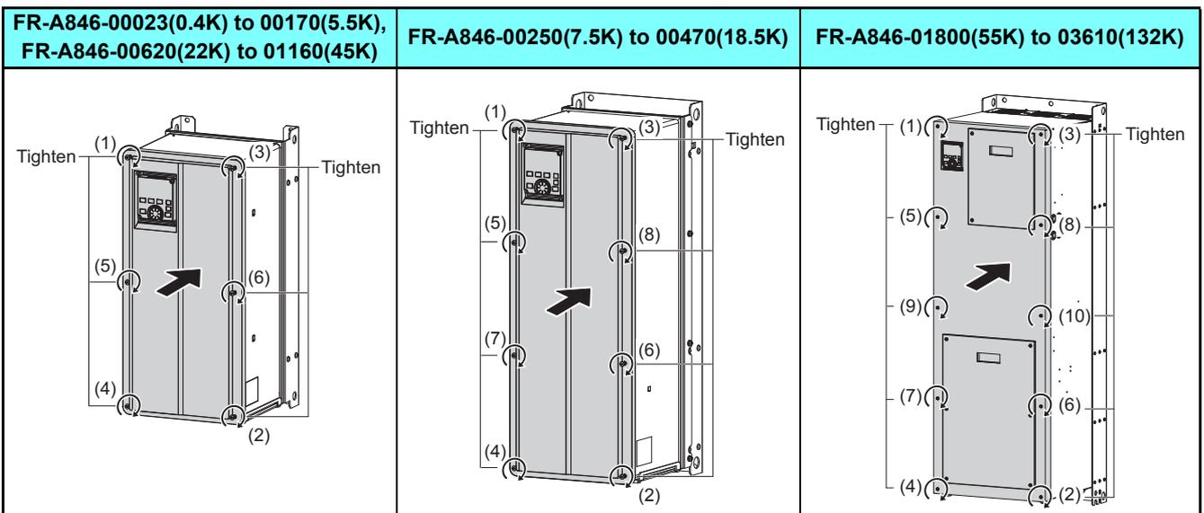
◆ **Removal of the front cover for control circuit inspection and the front cover for main circuit inspection (FR-A846-01800(55K) or higher)**
