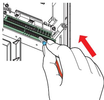
When using a single wire or stranded wires without a blade terminal, push the open/close button all the way down with a flathead screwdriver, and insert the wire.
