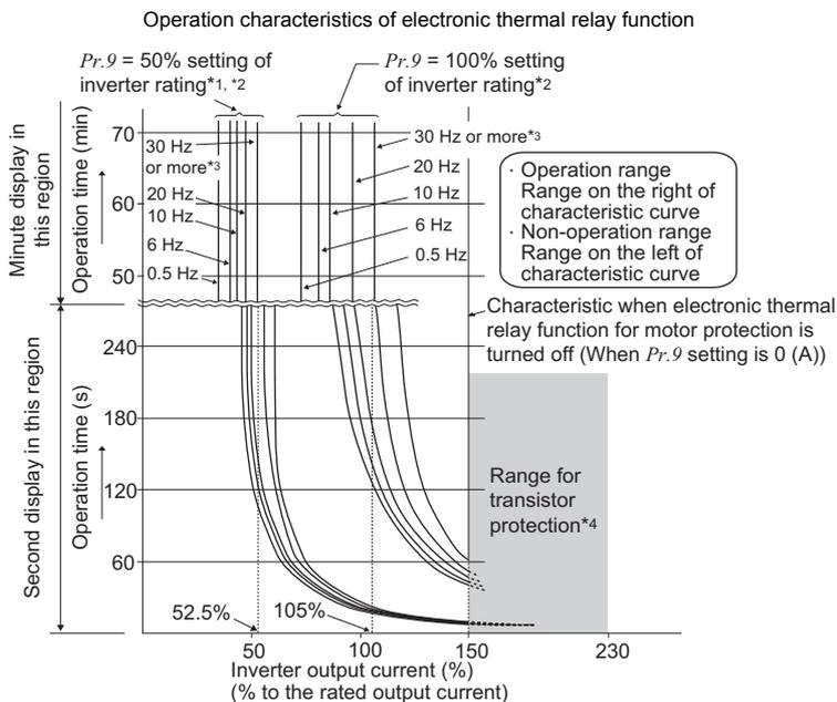
This function detects the overload of the motor, stops the operation of the inverter's output transistor, and stops the output. (The operation characteristic is shown on the left.)
