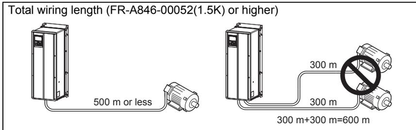
When driving a 400 V class motor by the inverter, surge voltages attributable to the wiring constants may occur at the motor terminals, deteriorating the insulation of the motor. In this case, take one of the following measures.
