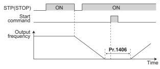
• When the output is shut off by the MRS signal, or when the inverter stops by a "0 Hz" frequency command while the start command is ON, the inverter output restarts even within the time set in **Pr.1406**.
