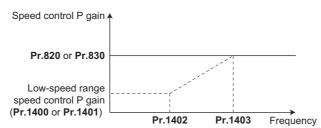
• When the value same as Pr.1403 setting and above is set in Pr.1402, the speed control P gain is as below.
