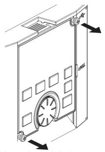
Push the upper part of the operation panel and pull the operation panel to remove.
