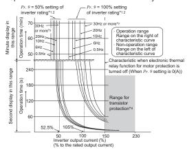
This function detects the overload (overheat) of the motor, stops the operation of the inverter's output transistor, and stops the output. (The operation characteristic is shown on the left.)
