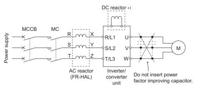
st 1 The converter unit (FR-CC2) is equipped with the DC reactor.
