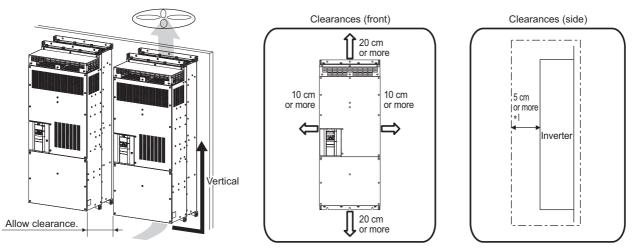
\*1 There needs to be a space of at least 30 cm in front of the inverter to replace the cooling fan. Refer to page 98 for fan replacement.
