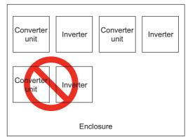
Arrangement of multiple inverters and converter units
