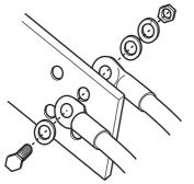
• When wiring the main circuit conductor (R/L1, S/L2, T/L3) of the converter unit (FR-CC2), use the bolts (nuts) for main circuit wiring, which are provided on the front side of the conductor.
