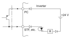
External signal input using transistor (source logic)
