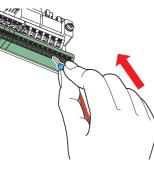
When using a single wire or stranded wires without a blade terminal, push the open/close button all the way down with a flathead screwdriver, and insert the wire.
