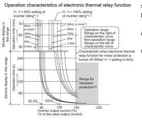
This function detects the overload (overheat) of the motor, stops the operation of the inverter's output transistor, and stops the output. (The operation characteristic is shown on the left.)
