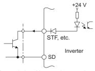
External signal input using transistor (sink logic)
