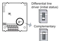
Terminating resistor selection switch (SW1)
