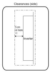
\*1 There needs to be a space of at least 30 cm in front of the inverter to replace the cooling fan. Refer to page 98 for fan replacement.
