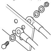
• When wiring the main circuit conductor (R/L1, S/L2, T/L3) of the converter unit (FR-CC2), use the bolts (nuts) for main circuit wiring, which are provided on the front side of the conductor.
