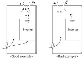
Arrangement of the ventilation fan and inverter
