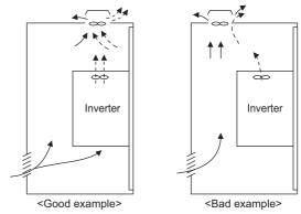
Arrangement of the ventilation fan and inverter
