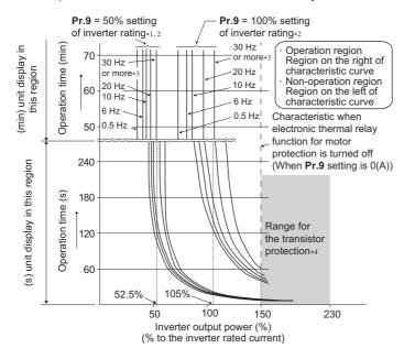
This function detects the overload (overheat) of the motor and trips the inverter by stopping the operation of the transistor at the inverter output side. (The operation characteristic is shown on the
