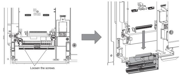
2) Be careful not to bend the pins of the inverter's control circuit connector, reinstall the control circuit terminal block and fix it with the mounting screws.
