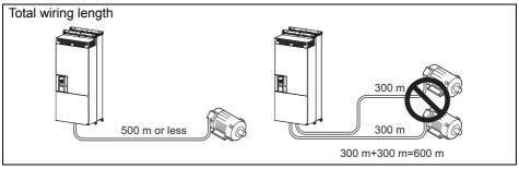
When driving a 400 V class motor by the inverter, surge voltages attributable to the wiring constants may occur at the motor terminals, deteriorating the insulation of the motor. In this case, take one of the following measure.
