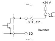
External signal input using transistor (sink logic)
