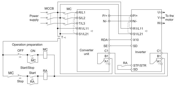
\*1 When the power supply is 400 V class, install a stepdown transformer.
