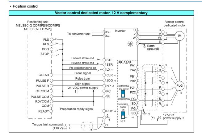
\*1 The pin number differs according to the encoder used. Speed, control, torque control, and position control by pulse train input are available with or without the Z-phase being connected
