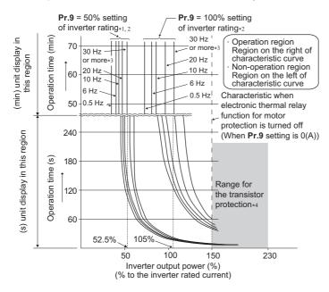
This function detects the overload of the motor and trips the inverter by stopping the operation of the transistor at the inverter output side. (The operation characteristic is shown on the left.)
