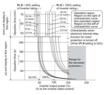
This function detects the overload (overheat) of the motor and trips the inverter by stopping the operation of the transistor at the inverter output side. (The operation characteristic is shown on the left.)
