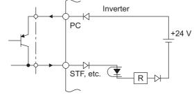
External signal input using transistor (source logic)
