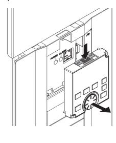
To reinstall the operation panel, align its connector on the back with the PU connector of the inverter, and insert the operation panel. After confirming that the operation panel is fit securely, tighten the screws. (Tightening torque: 0.40 to 0.45 N·m)
