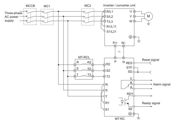
\*1 For the FR-A842-08660(355K) or lower, up to two cables can be connected to terminals P/+ and N/-. For the FR-A842-09620(400K) or higher, up to four cables can be connected. To use more cables, use a bus bar.
