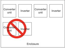
Arrangement of multiple inverters and converter units
