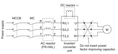
\*1 The converter unit (FR-CC2) is equipped with the DC reactor.
