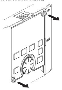
Press the upper edge of the operation panel while pulling out the operation panel.
