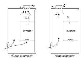
Arrangement of the ventilation fan and inverter
