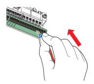
When using single wire or stranded wire without crimp terminal, push an open/close button all the way down with a flathead screw driver, and insert the wire.
