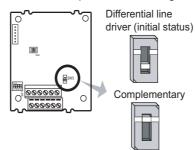
Use the terminating resistor selection switches (SW1) to select ON/OFF of the internal terminating resistor.
