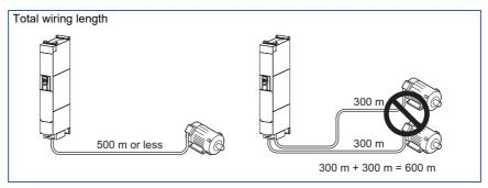
When driving a 690 V class motor by the inverter, surge voltages attributable to the wiring constants may occur at the motor terminals, deteriorating the insulation of the motor. In this case, use a 690 V class inverter-driven insulation-enhanced motor. When the wiring length exceeds 100 m, set "4" (4 kHz) or less in **Pr.72 PWM frequency selection** (carrier frequency).
