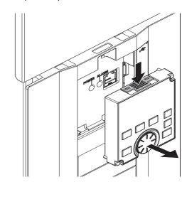
To reinstall the operation panel, align its connector on the back with the PU connector of the inverter, and insert the operation panel. After confirming that the operation panel is fit securely, tighten the screws. (Tightening torque: 0.40 to 0.45 N·m)
