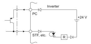
External signal input using transistor (source logic)
