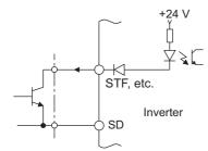
External signal input using transistor (sink logic)
