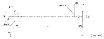
\*1 The bus bar dimensions differ depending on the arrangement of the inverter and the converter unit as shown in the following table.
