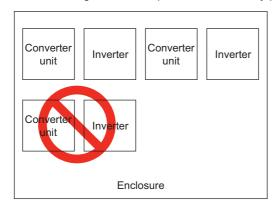
Arrangement of multiple inverters and converter units
