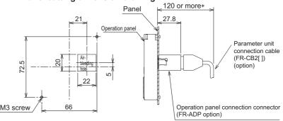
\* Denotes the space required to connect an optional parameter unit connection cable (FR-CB2[]). When using another cable, leave the space required for the cable specification.
