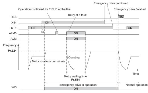
The following diagram shows the operation of switching over to the commercial power supply operation during emergency drive operation by using the CS signal (in the commercial mode or in the fixed frequency mode (Pr.523 = "411")).
