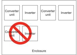
Arrangement of multiple inverters and converter units
