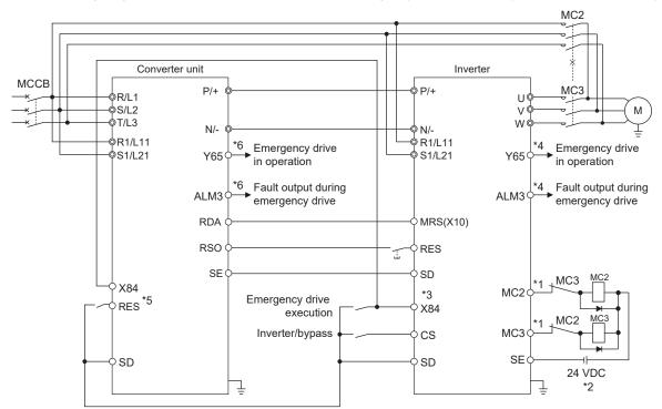
\*1 Be careful of the capacity of the sequence output terminals. The applied terminals differ by the settings of **Pr.190 to Pr.196 (Output terminal function selection)**.
