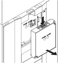
To install the accessory cover, fit it securely and tighten the screws. (Tightening torque: 0.40 to 0.45 N·m)
