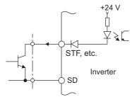
External signal input using transistor (sink logic)
