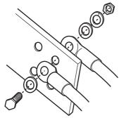
• When wiring the main circuit conductor (terminals R/L1, S/L2, T/L3) of the converter unit (FR-CC2-C), use the bolts (nuts) for main circuit wiring, which are provided on the front side of the conductor.
