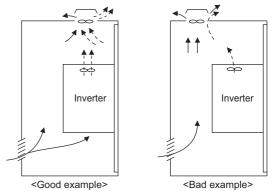
Arrangement of the ventilation fan and inverter
