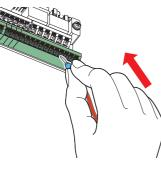
When using single wire or stranded wires without a crimp terminal, push the open/close button all the way down with a flathead screwdriver, and insert the wire.
