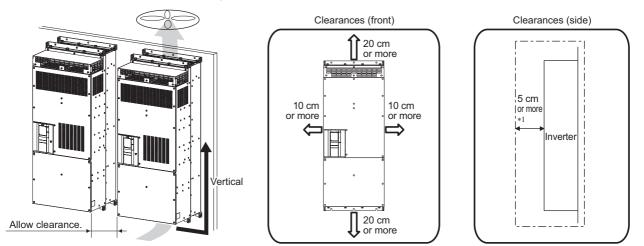
\*1 For replacing the cooling fan, 30 cm or more of space is necessary in front of the inverter. Refer to page 72 for fan replacement.
