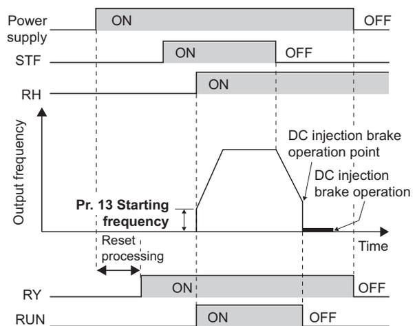
(c) Checking the inverter operating status by the start signal input to the inverter and inverter running signal
