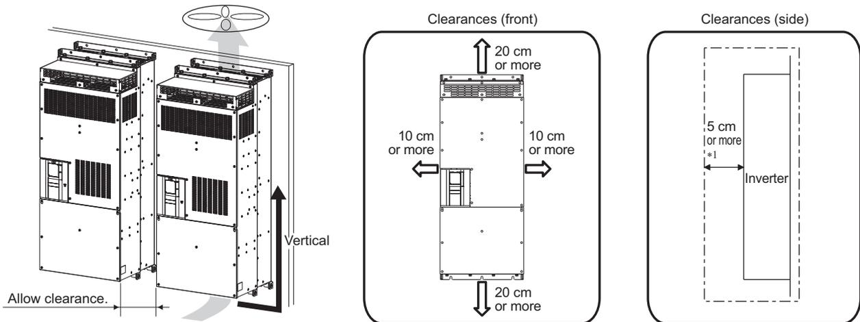
\*1 For replacing the cooling fan, 30 cm or more of space is necessary in front of the inverter. Refer to [page 76](#) for fan replacement.
