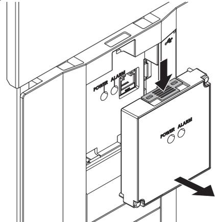
To install the accessory cover, fit it securely and tighten the screws. (Tightening torque: 0.40 to 0.45 N·m)
