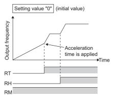
• Turning ON the RT signal enables the second function, and turning ON the X9 signal enables the third function. The following table shows the functions which can be changed to the second or third function.
