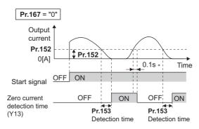
\* When the output is restored to the **Pr.152** level, the Y13 signal is turned OFF after 0.1 s.
