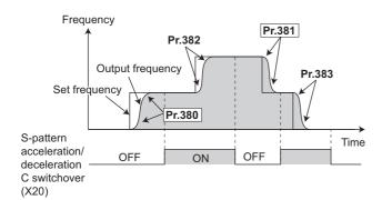
• Set the ratio (%) of time for drawing an S-shape in Pr.380 to Pr.383 with the acceleration time as 100%.
