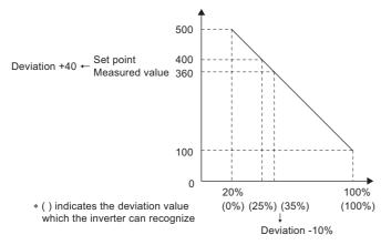
The display of the following parameters is changed according to the C42 (Pr.934)), C44 (Pr.935), Pr.1136, and Pr.1138 settings.
