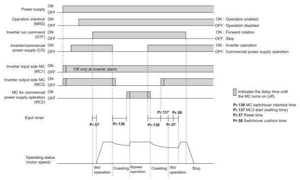
• Example of operation sequence with automatic bypass sequence (Pr.139 ≠ "9999", Pr.159 = "9999")
