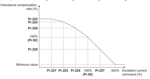
Setting example when Pr.225 setting < Pr.223 setting < Pr.221 setting < Pr.227 setting</li>
