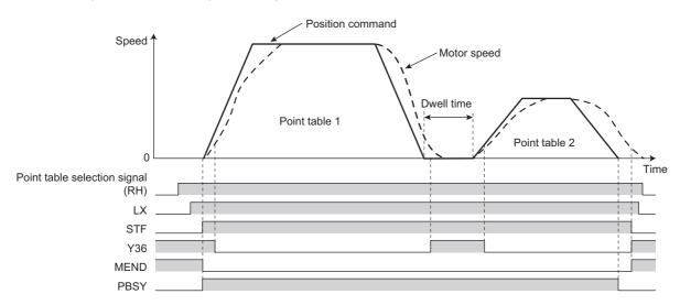
• Output signal operation during positioning with home position return
