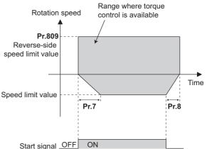
When the torque command value is negative
