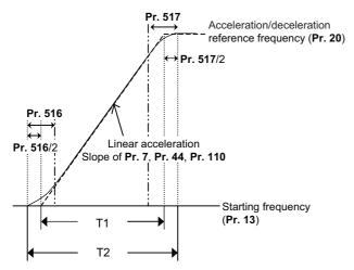
Set acceleration time T1 = (set frequency - Pr.13) × Pr.7 / Pr.20
