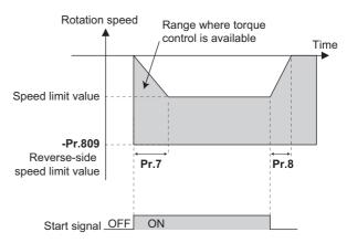
For regenerative driving by reverse rotation command (unwinding)
