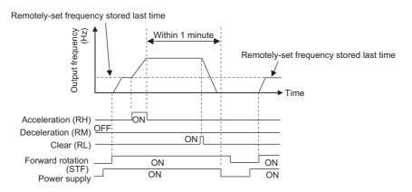
• When the remotely-set frequency is cleared by turning ON the RL (clear) signal after turning OFF (ON) both the RH and RM signals, the inverter operates at the frequency in the remotely-set frequency cleared state if power is reapplied before one minute has elapsed since turning OFF (ON) both the RH and RM signals.
