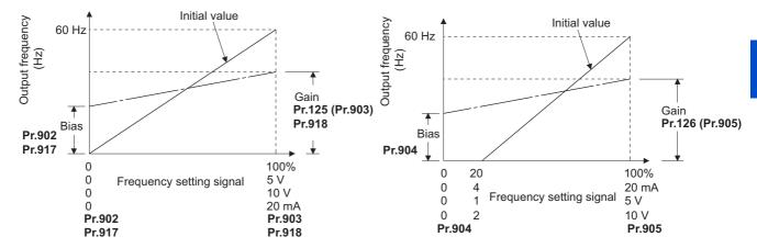
There are three methods to adjust the frequency setting voltage (current) bias/gain.
