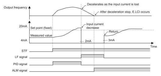
• The following is the operation example when the analog input current is restored during deceleration under PID control (reverse action).
