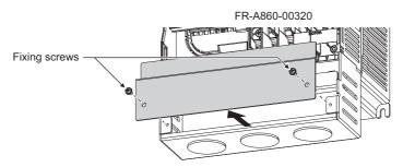
**3.** Loosen the fixing screws that fix the wiring cover to the inverter, and remove the wiring cover.
