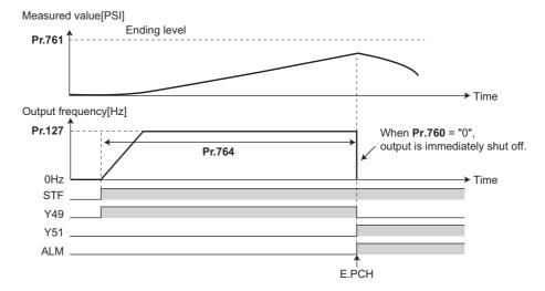
• Example of protective function measured value limit (Pr.760 = "1")
