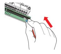
When using a single wire or stranded wires without a crimp terminal, push the open/close button all the way down with a flathead screwdriver, and insert the wire.
