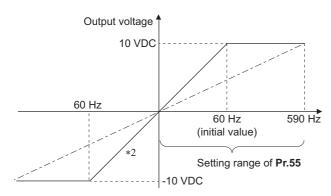
\*1 Output with a negative sign available when **Pr.290 Monitor negative output selection** = "1, 3"
