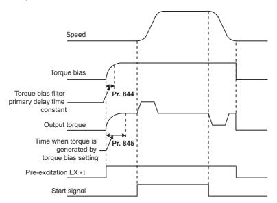
\*1 When pre-excitation is not performed, the torque bias functions at the same time as the start signal.
