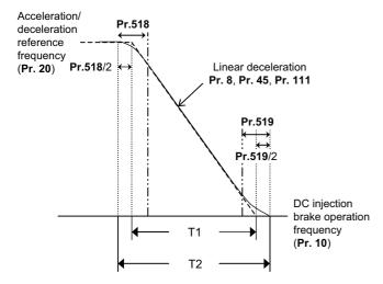
Set deceleration time T1 = (set frequency - Pr.10 DC injection brake operation frequency)  $\times$  Pr.8 / Pr.20 = (60 Hz - 3 Hz)  $\times$  5 s / 60 Hz  $\stackrel{.}{=}$  4.75 s (actual deceleration time at linear deceleration) Actual deceleration time T2 = set deceleration time T1 + (Pr.518 + Pr.519) / 2 = 4.75 s + (0.1 s + 0.1 s) / 2 = 4.85 s (deceleration time at S-pattern deceleration)
