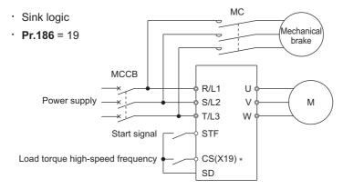
\*1 The applied terminals differ by the settings of Pr.180 to Pr.189 (Input terminal function selection).
