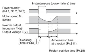
\* The output shut off timing differs according to the load condition.
