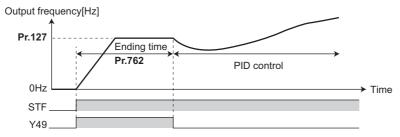
· When the signal is input to end the pre-charge operation
