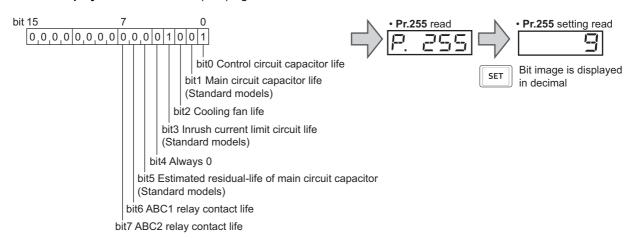
• When the parts have reached the life alarm output level, the corresponding bits of **Pr.255** turns ON. The ON/OFF state of the bits can be checked with **Pr.255**. The following table shows examples.
