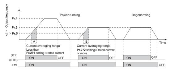
• When the average current is larger than "inverter rated current × **Pr.271** setting (%)" and smaller than "inverter rated current × **Pr.272** setting (%)", linear compensation is performed as shown below.
