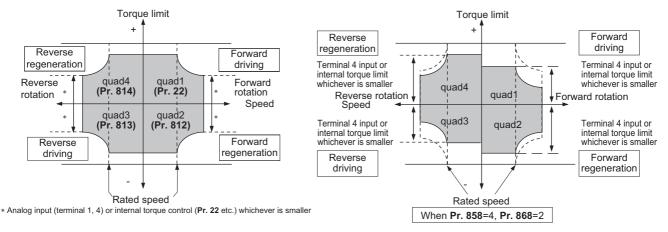
• The torque limit using analog input can be corrected with Calibration parameters Pr.919, Pr.920, Pr.932, and Pr.933. (Refer to page 488.)
