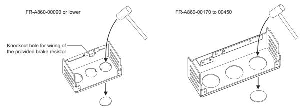
**2.** Conduit hubs must always be used to connect conduit to the enclosure knockout. The hub shall be assembled to the conduit before it is installed in the conduit box knockout opening.
