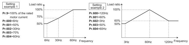
When setting Pr.600, Pr.602, Pr.604 (Pr.692, Pr.694, Pr.696) to the same frequency, the following graph's upper level will be applied.
