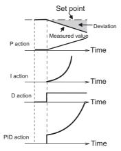
(Note) PID action is the result of all P, I and D actions being added together.
