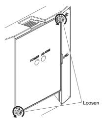
2. Press the upper edge of the accessory cover while pulling out the accessory cover.
