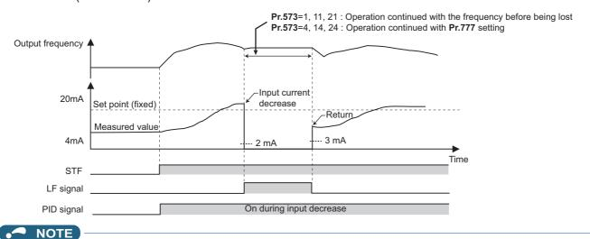
• When the setting is changed to continuously operate after the input current loss (**Pr.573** = "1, 4, 11, 14, 21, or 24"), the motor will operate as the frequency before loss is 0 Hz.
