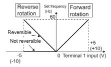
Compensation input characteristics when STF is ON
