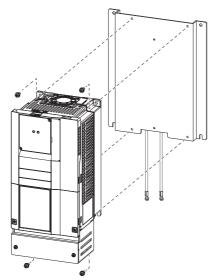
**3.** Make cuts in the provided protective bush with a nipper, a cutter knife, etc. and attach it to the knockout hole on the wiring cover for wiring the provided brake resistor. Connect the provided brake resistor cable with red sleeve to terminal PR, and the cable with transparent sleeve to terminal P3. (For details on the terminals PR and P3, refer to page 43.)
