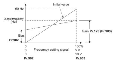
Other adjustment methods for the frequency setting voltage gain are the following: adjustment by applying a voltage directly across terminals 2 and 5, and adjustment using a specified point without applying a voltage across terminals 2 and 5.
