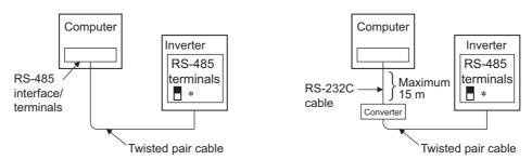
\*Set the terminating resistor switch to the " $100\Omega$ " position.
