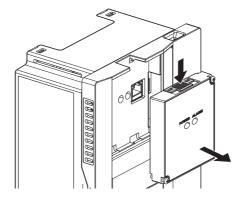
To install the accessory cover, fit it securely and tighten the screws. (Tightening torque: 0.40 to 0.45 N·m)
