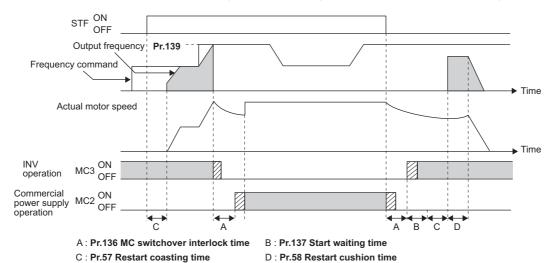
• Example of operation sequence with automatic bypass sequence (Pr.139 ≠ "9999", Pr.159 ≠ "9999")
