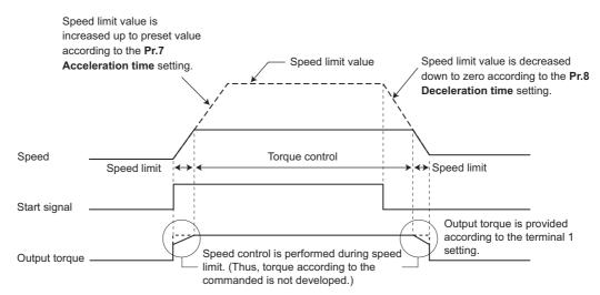
• If the setting value of **Pr.7 and Pr.8** is "0", turning OFF the start signal enables speed control, and the output torque is controlled by the torque limit value.
