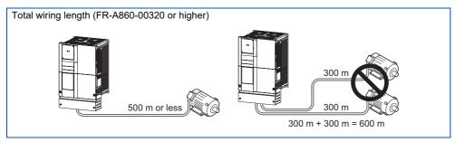
• When fast response current limit is enabled (**Pr.156** = "0, 2, 4, 6, 8, 10, 12, 14, 16, 18, 20, 22, 24, 26, 28, or 30"), the wiring length should be within the value in the table below.
