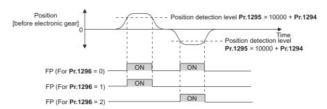
When a current position varies, the position detected signal may repeat ON/OFF (chatter). Setting hysteresis to the
