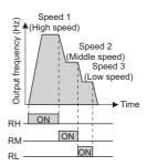
The following shows the procedure to operate at a high-speed (60 Hz).
