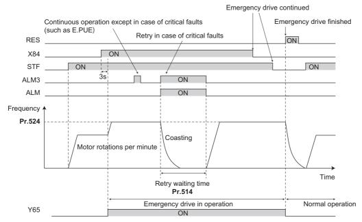
• The following diagram shows the operation of switching over to the commercial power supply operation during emergency drive operation by using the CS signal (in the commercial mode or in the fixed frequency mode (**Pr.523** = "411")).
