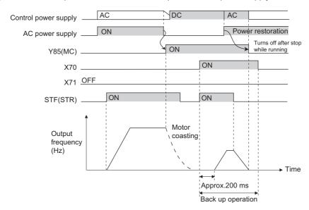
· Operation example at the time of power failure occurrence 3 (when continuing the operation)
