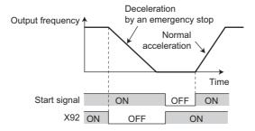
• The droop control and the speed loop integration at the emergency stop by the Emergency stop (X92) signal can be enabled/disabled using **Pr.1349 Emergency stop operation selection**.
