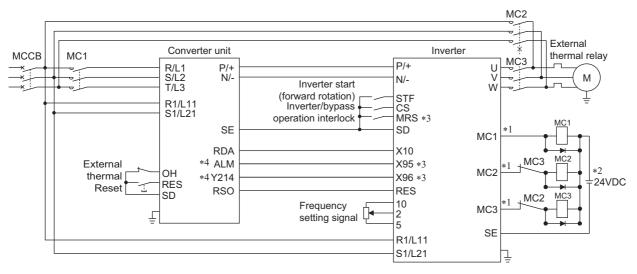
\*1 Be careful of the capacity of the sequence output terminals. The applied terminals differ by the settings of Pr.190 to Pr.196 (Output terminal function selection).
