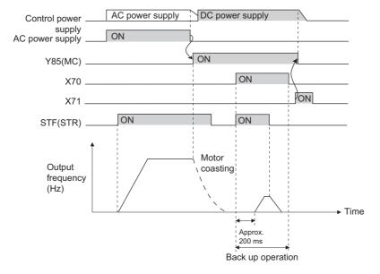
· Operation example at the time of power failure occurrence 2 (when the AC power supply is restored)
