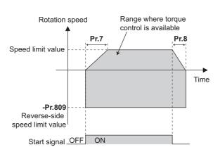
When the torque command value is positive
