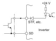
External signal input using transistor (sink logic)
