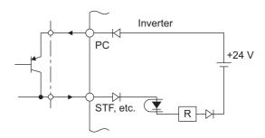
External signal input using transistor (source logic)
