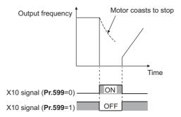
· Relationship between Pr.599 and the inverter operation enable signal of each option unit
