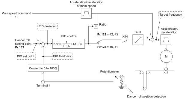
11 The main speed can be selected in all operation modes, External (analog voltage input, multi-speed), PU (digital frequency setting) and Communication (RS-485).
