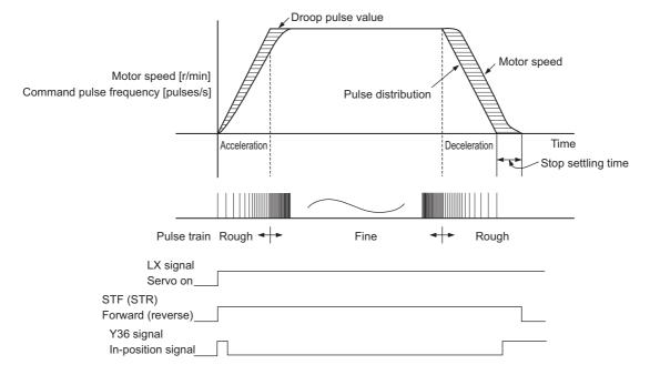
• The pulses are slow during motor acceleration. The pulses are fast at full speed. The pulses become slower during deceleration, and eventually becomes 0 and the motor stops a little after the command pulse. This time difference is necessary to ensure stop accuracy and is called stop setting time.
