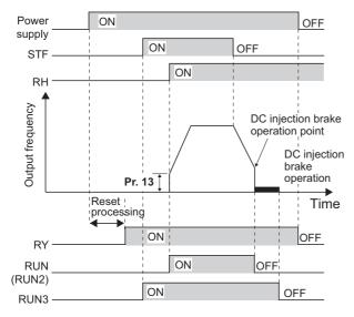
· According to the inverter condition, the ON/OFF operation of each signal is as shown below.
