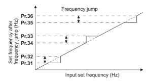
• [Example 1] To fix the frequency to 30 Hz in the range of 30 Hz to 35 Hz, set 35 Hz in Pr.34 and 30 Hz in Pr.33.
