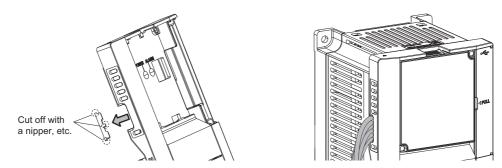
• When the FR-A860-00680 or higher is used with a plug-in option, lead the wires on the left side of the plug-in option for wiring of the RS-485 terminals.
