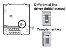
· Terminating resistor selection switch (SW1)
