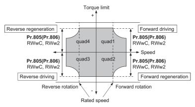
• When the CC-Link communication (Ver. 2) is used in the quadruple or octuple setting (**Pr.544**="24, 28, or 128"), the torque limit value can be input using a remote register (RWwC to RWwF) for each of the four quadrants.
