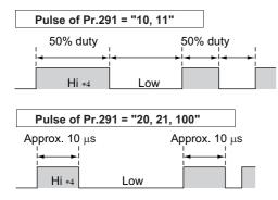
\*4 "HIGH" indicates when the open collector output transistor is OFF.
