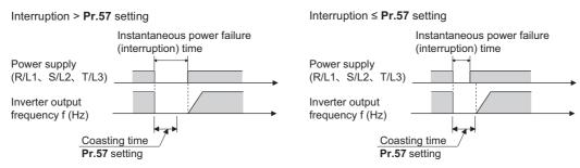
• Inverter operation is sometimes hindered by the size of the moment of inertia (J) of the load, output frequency, or the residual magnetic flux in the motor. Adjust this coasting time within the range 0.1 to 30 seconds to match the load specification.
