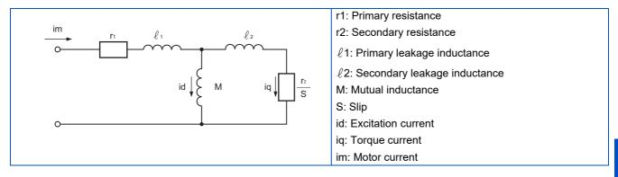
In the above diagram, currents flowing in the induction motor can be classified into a current id (excitation current) for making a magnetic flux in the motor and a current iq (torque current) for causing the motor to develop torque.
