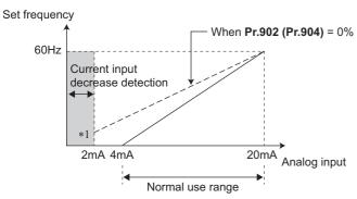
\*1 When the **Pr.573** ≠ "9999" and terminal 4 (terminal 2) is calibrated to 2 mA or less with **Pr.902** (**Pr.904**), analog input frequency that is 2 mA or less will become input current loss, thus it will not be as the bias setting frequency.
