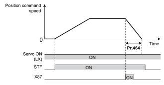
• The input logic of the X87 signal can be set using Pr.1292 Position control terminal input selection.
