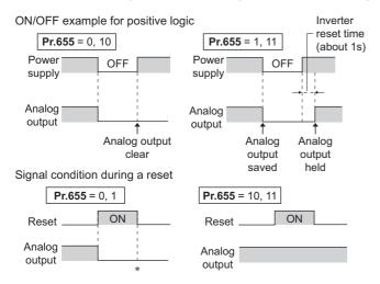
\* When **Pr.655** = "1", the signal condition saved in EEPROM (condition of the last power OFF) is applied.
