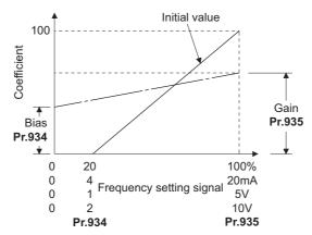
• There are three methods to adjust the PID display bias/gain.
