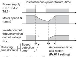
\* The output shut off timing differs according to the load condition.
