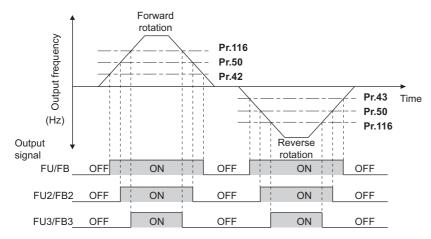
• For each signal, refer to the following table and assign the function by **Pr.190 to Pr.196 (Output terminal function selection)**.
