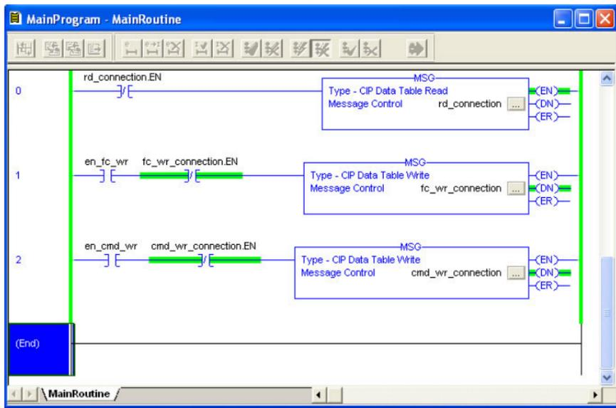
**Figure 51: Reading and Writing via MSG Instructions**
