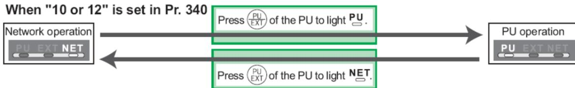
For a switching method via external terminal input signals, refer to the inverter's *user's manual (applied)*.
