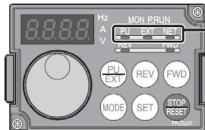
Operation mode indication (the inverter operates in accordance with the indicated LED.)
