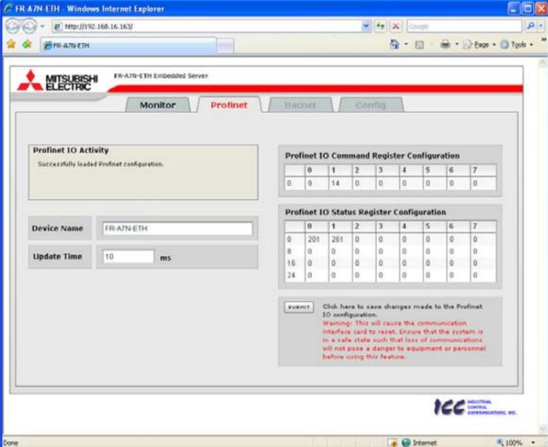
The screenshot shows the Profinet configuration page for the FR-A7N-ETH Embedded Server. The page is viewed in Internet Explorer at the URL http://192.168.16.163/. The interface includes a navigation bar with tabs for Monitor, Profinet (selected), Backet, and Config. The main content area is divided into several sections:
