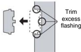
Remove front cover wiring access knockout and trim any excess flashing that may cause cable damage
