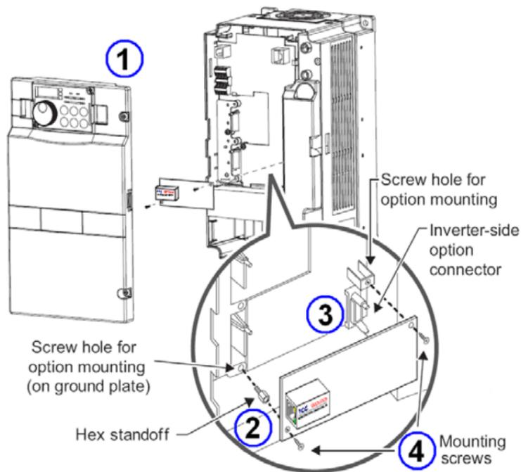
1) Remove the inverter's front cover.
