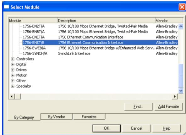
Figure 35: Adding a New Module
