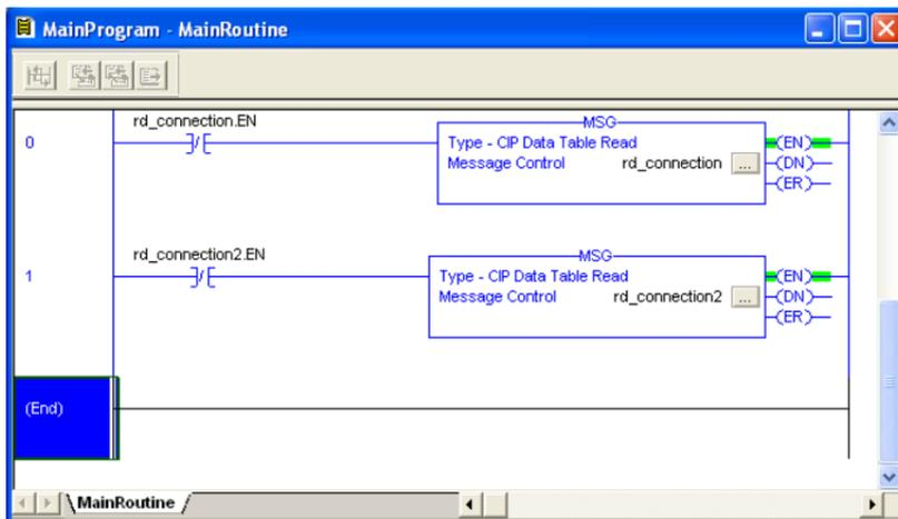
Figure 50: Reading Via Multiple MSG Instructions
