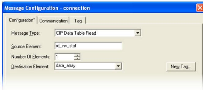
**Figure 49: Read the Inverter's Status Register**
