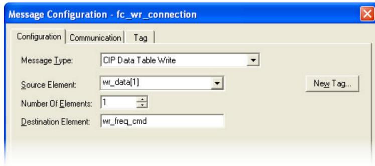
**Figure 52: MSG Configuration for Writing**
