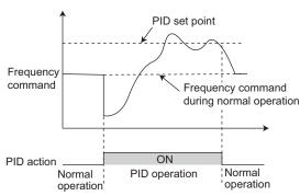
Operation when control is switched to PID control during normal operation
