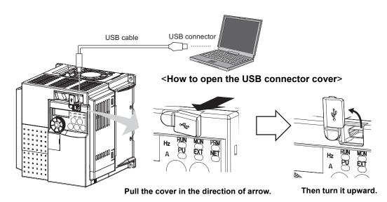
· You can perform parameter setting and monitoring with the FR Configurator. Refer to the instruction manual of the FR Configurator for details.
