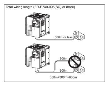
When driving a 400V class motor by the inverter, surge voltages attributable to the wiring constants may occur at the motor terminals, deteriorating the insulation of the motor. (Refer to page 92)
