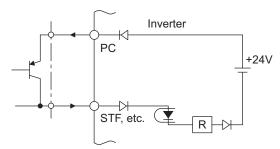
External signal input using transistor
