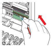
When using a single wire or stranded wire without a blade terminal, push an open/close button all the way down with a flathead screw driver, and insert the wire.
