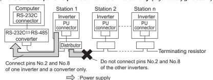
Do not connect the PU connector to the computer's LAN board, FAX modem socket or telephone modular connector.
