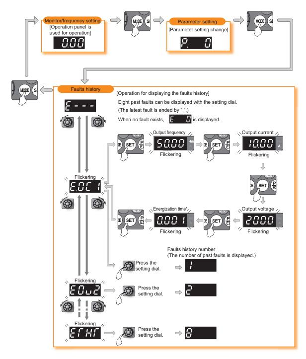
\* The cumulative energization time and actual operation time are accumulated from 0 to 65535 hours, then cleared, and accumulated again from 0. When the operation panel is used, the time is displayed up to 65.53 (65530h) in the indication of 1h = 0.001, and thereafter, it is added up from 0.
