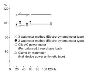
Example of **Measuring Inverter Input Power**
