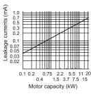
Ig1, Ig2: Leakage currents in wire path during commercial power supply operation
