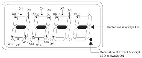
•On the output option terminal monitor (Pr. 52 = "57"), the decimal point LED of the second digit LED is ON.
