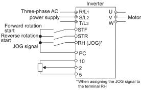
Connection diagram for external Jog operation
