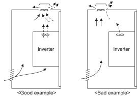
Placement of ventilation fan and inverter
