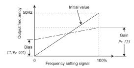
•When ratio ( $Pr.\ 128$  = "42, 43") is selected for addition method, PID control × (ratio of main speed) is added to the main speed. The ratio is determined by the  $Pr.\ 125$  Terminal 2 frequency setting gain frequency and C2 ( $Pr.\ 902$ ) Terminal 2 frequency setting bias frequency. The frequency setting signal is set to 0 to 50Hz in the range between 0 to 100% in the initial setting. The ratio is (×100%) when the main speed is 50Hz and (×50%) when 25Hz.
