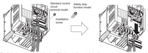
(2) Using care not to bend the pins of the inverter's control circuit connector, reinstall the control circuit terminal block and fix it with the installation screw.
