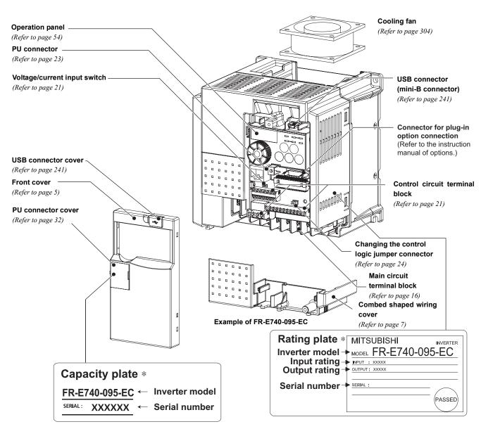
Location of the capacity plate and the rating plate differs according to the inverter capacity.
