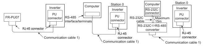
● Combination of a computer and multiple inverters (1:n connection)
