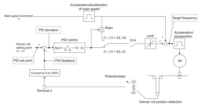
\*1 The main speed can be selected from all operation mode such as external (analog voltage input, multi-speed), PU (digital frequency setting), communication (RS-485, CC-Link).
