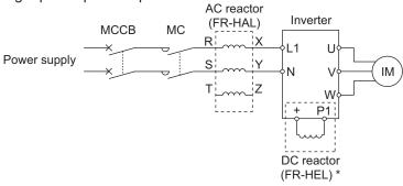
\* When connecting the FR-HEL, remove the jumper across terminals P/+ and P1.
