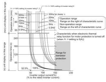
This function detects the overload (overheat) of the motor and trips. (The operation characteristic is shown on the left)
