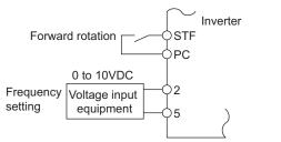
Connection diagram using terminal 2 (0 to 10VDC)
