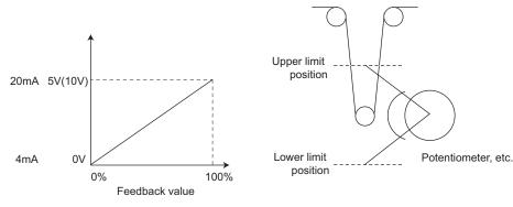
(Example) Control at a dancer center position using a 0 to 7V potentiometer
