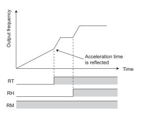
• When the RT signal is ON, the following second function is selected at the same time.
