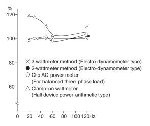
Example of **Measuring Inverter Output Power**
