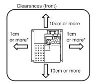
\* When using the inverters at the surrounding air temperature of 40 °C or less, the inverters can be installed without any clearance between them (0cm clearance).
