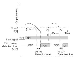
\* The zero current detection signal (Y13) holds the signal for approximately 100ms once turned ON.
