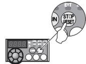
Operation 2: ..... Turn ON the reset signal (RES) for more than 0.1s. (If the RES signal is kept ON, "Err." appears (flickers) to indicate that the inverter is in a reset status.)
