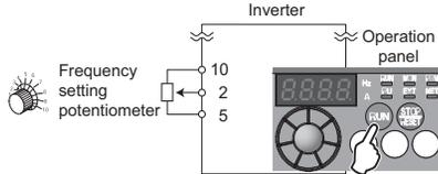
Operation example Operate at 60Hz.
