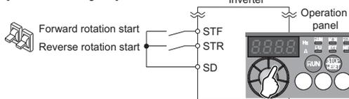
Operation example Operate at 30Hz.
