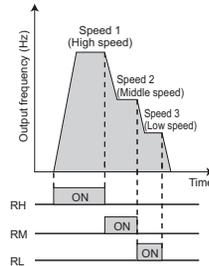
Operation example    Operation at low speed (10Hz)
