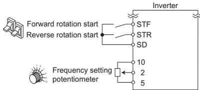
**Operation example** Operate at 60Hz.
