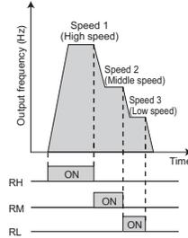
Operation example    Operation at high speed (60Hz)
