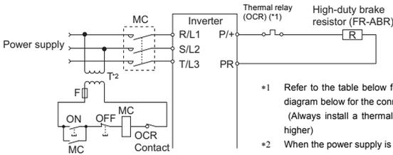
\*1 Refer to the table below for the type number of each capacity of thermal relay and the diagram below for the connection.
