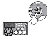
Operation 2: ..... Change the error reset signal setting of the FL remote communication from "0" to "1."
