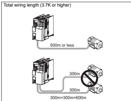
When driving a 400V class motor by the inverter, surge voltages attributable to the wiring constants may occur at the motor terminals, deteriorating the insulation of the motor. Take the following measures (1) or (2) in this case.
