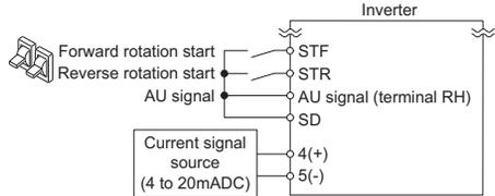
Operation example Operate at 60Hz.
