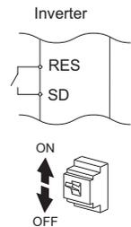
Operation 3 ..... Switch power OFF once. After the indicator of the operation panel turns OFF, switch it ON again.
