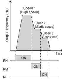
Operation example    Operation at high speed (60Hz)
