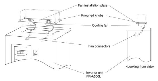
Caution: The number of cooling fans used differs according to the inverter capacity. Depending on the number of cooling fans used, they may be installed on two installation plates.
