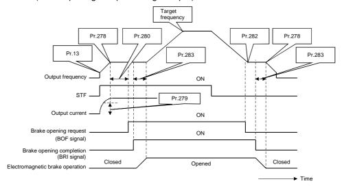
2) Pr. 60 = "8" (mechanical brake opening completion signal not input)
