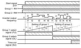
(7) To repeat the operation of the same group, reset the timer using the time-out signal as shown below.
