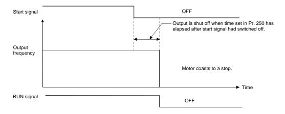
Note: 1. The RUN signal switches off when the output stops.
