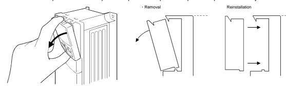
To reinstall, insert straight and mount securely.
