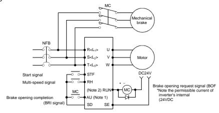
Note: 1. The input signal terminal used depends on the Pr. 180 to Pr. 186 settings.
