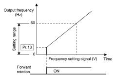
Note: The inverter will not start if the frequency setting signal is less than the value set in Pr. 13 "starting frequency".
