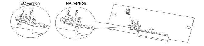
3) Using care not to bend the pins of the control circuit connector, reinstall the control circuit terminal block and fix it with the mounting screws.
