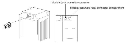
3) Securely plug one end of the connection cable into the PU connector (modular jack type relay connector) of the inverter and the other end into the operation panel. (Refer to page 19)
