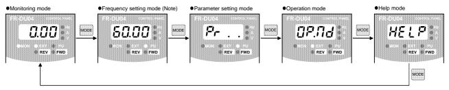
Note: The frequency setting mode is displayed only in the PU operation mode.
