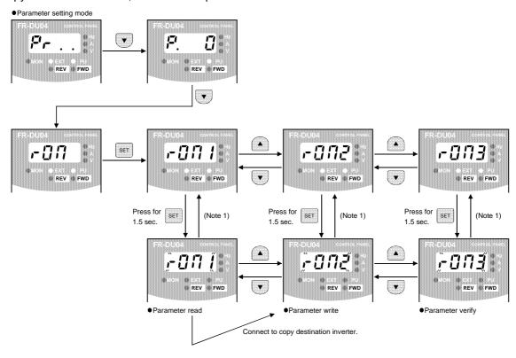
Note: 1. While the copy function is being activated, the monitor display flickers. The display returns to the lit-up state on completion of the copy function.
