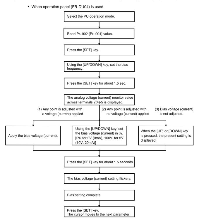
\*Pr. 903 to Pr. 905 can also be adjusted similarly using the above procedure.
