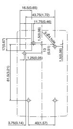
PU connector pin layout (Looking from front of inverter unit "receptacle side")
