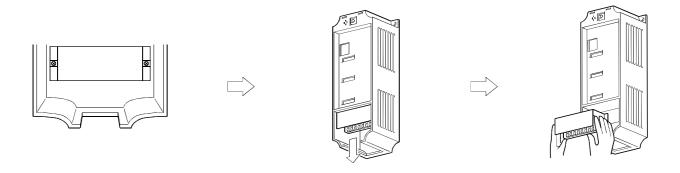
2) Remove the connector in the sink logic position on the back surface of the control circuit terminal block and fit it to the source logic position.
