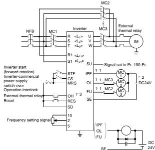
Note: This switch-over function is used in the external operation mode. Always connect terminals R1, S1 to a different power (power supply different from the one for MC1) to ensure operation
