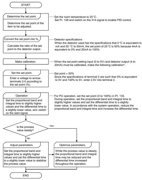
\*When calibration is required, use Pr. 902 to Pr. 905 to calibrate the detector output and set point setting input in the PU mode during an inverter stop.
