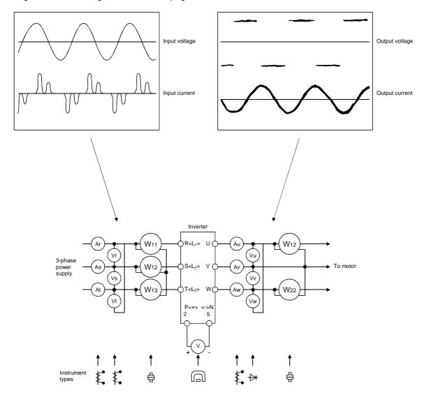
**Typical Measuring Points and Instruments**
