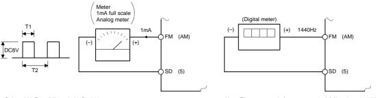
Pulse width T1 :Adjusted with Pr. 900
