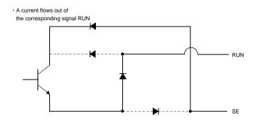
When using an external power supply for transistor output, use terminal SD as a common to prevent misoperation caused by leakage current.
