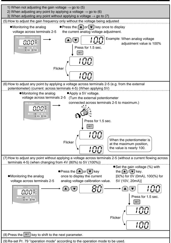
Note: 1. If the Pr. 903 or Pr. 905 (gain adjustment) value is changed, the Pr. 20 value does not change.
