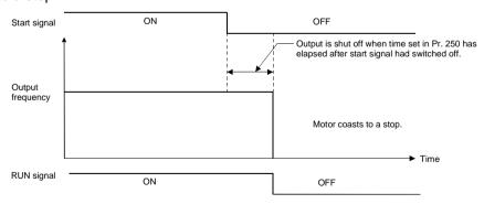
Note: 1. The RUN signal switches off when the output stops.
