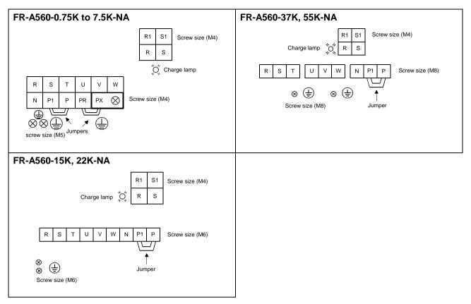
Note: 7.5K does not have the jumper across the terminals PR-PX.
