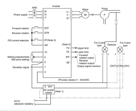
Note: 1. The power supply must be selected in accordance with the power specifications of the detector used.
