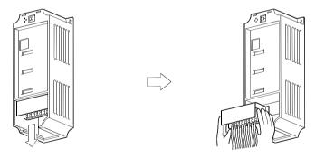
3) When installing the terminal block to a new inverter, exercise care not to bend the pins of the control circuit terminal block connector.
