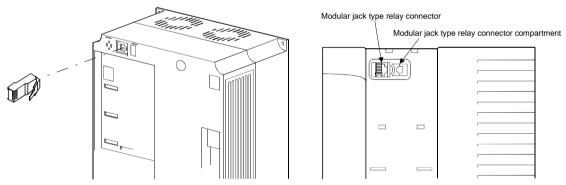
3) Securely plug one end of the connection cable into the PU connector (modular jack type relay connector) of the inverter and the other end into the operation panel.
