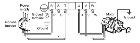
The power supply cables must be connected to R, S, T. If they are connected to U, V, W, the inverter will be damaged. Phase sequence need not be matched.
