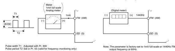
• Terminal AM is factory-set to provide a 10VDC output in the full-scale state of each monitored data. Pr. 901 allows the output voltage ratio (gain) to be adjusted according to the meter reading. Note that the maximum output voltage is 10VDC.
