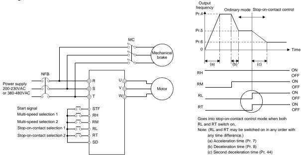
Note: The input signal terminals used depend on the Pr. 180 to Pr. 186 settings.
