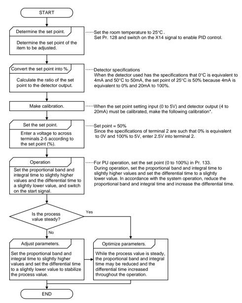
\*When calibration is required, use Pr. 902 to Pr. 905 to calibrate the detector output and set point setting input in the PU mode during an inverter stop.
