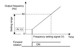
Note: The inverter will not start if the frequency setting signal is less than the value set in Pr. 13 "starting frequency".
