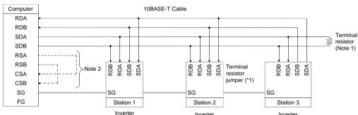
Note: 1. There may be the influence of reflection depending on the transmission speed and/or transmission distance. If this reflection hinders communication, provide a terminal resistor. If the PU connector is used to make a connection, use a distributor as a terminal resistor cannot be fitted. Connect the terminal resistor only to the inverter remotest from the computer.(Terminal resistor:  $100~\Omega$ )
