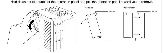
To reinstall, insert straight and mount securely.
