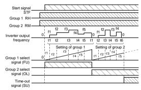
(7) To repeat the operation of the same group, reset the timer using the time-out signal as shown below.
