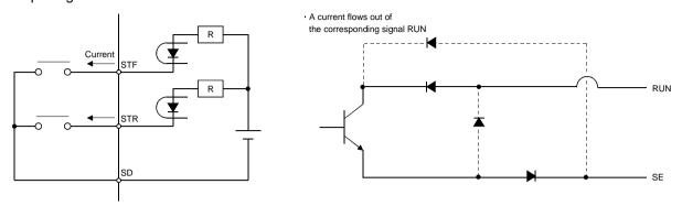
When using an external power supply for transistor output, use terminal PC as a common to prevent misoperation caused by leakage current. (Do not connect terminal SD of the inverter with terminal 0V of the external power supply.)
