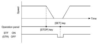
(Example) A restart after a stop during external operation
