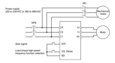
Note: The input signal terminal used depends on the Pr. 180 to Pr. 186 settings.
