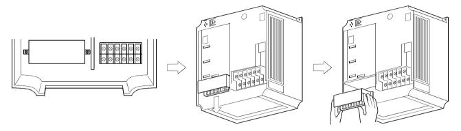
2) Remove the connector from the rear surface of the control circuit terminal block and place in required Logic position (either Sink or Source).
