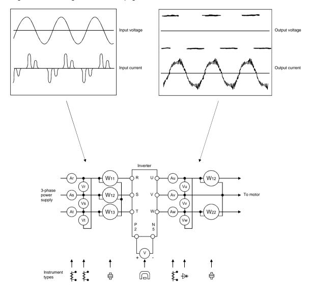
**Typical Measuring Points and Instruments**
