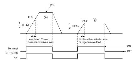
When operation is performed with X19 (load detection high-speed frequency function selection) signal on, the inverter automatically varies the maximum frequency between Pr. 4 "multi-speed setting (high speed)" and Pr. 5 "multi-speed setting (middle speed)" settings as shown below according to the average current flowing during acceleration from the frequency half of the Pr. 5 setting to the frequency set in Pr. 5.
