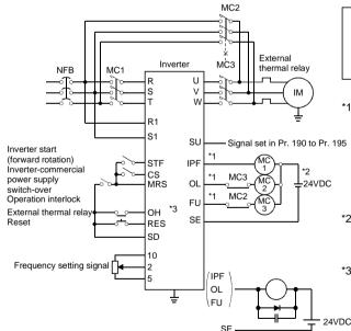
Note: This switch-over function is used in the external operation mode. Always connect terminals R1, S1 to a different power supply (power supply different from the one for MC1) to ensure proper operation.
