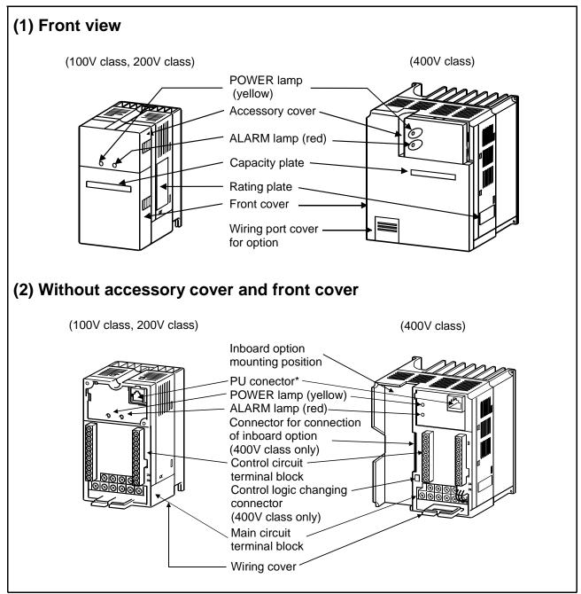
\*Use the PU connector for the FR-PA02-02 or FR-PU04 option and RS-485 communication.
