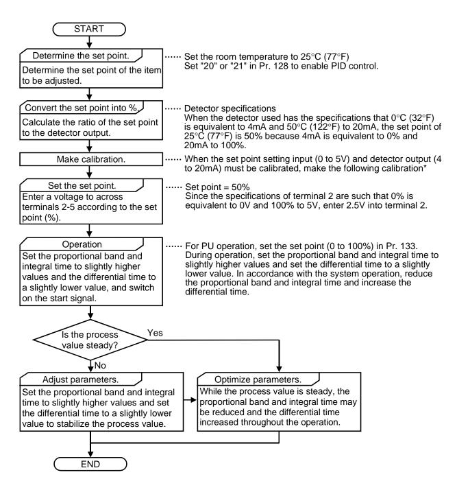
\* When calibration is required, use Pr. 902 to Pr. 905 to calibrate the detector output and set point setting input in the PU mode during an inverter stop.
