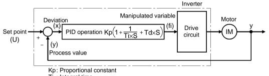
Ti: Integral time S: Operator Td: Differential time
