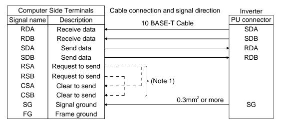
2) Wiring of one RS-485 computer and "n" inverters (several inverters)
