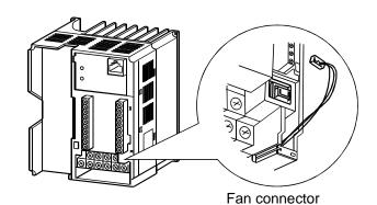
3) Remove the inverter and cooling fan.
