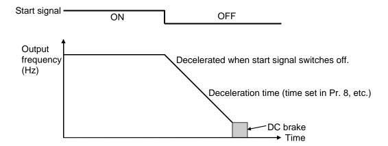
(2) Pr. 250 = 0 to 100 seconds (output is shut off after preset time)
