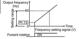
Note: The inverter will not start if the frequency setting signal is less than the value set in Pr. 13 "starting frequency".
