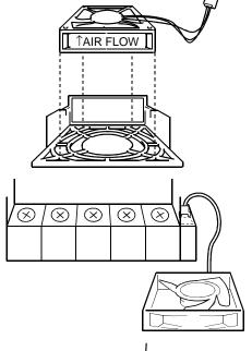
2) Reinstall the fan cover to the inverter.
