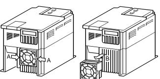
4) Remove the cooling fan and cooing fan cover.
