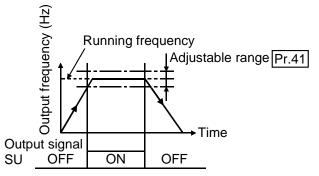
• Use any of Pr. 190 to Pr. 192 to allocate the terminal used for SU signal output. Refer to page 150 for Pr. 190 to Pr. 192 (output terminal function selection).
