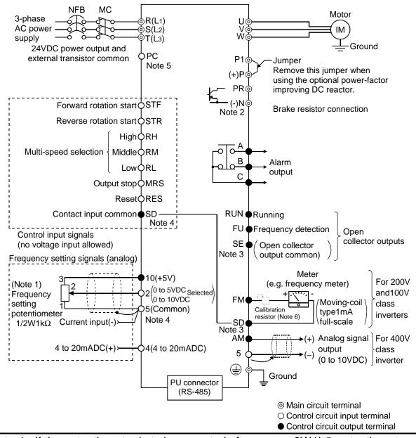
Note: 1. If the potentiometer is to be operated often, use a  $2W1k\Omega$  potentiometer.
