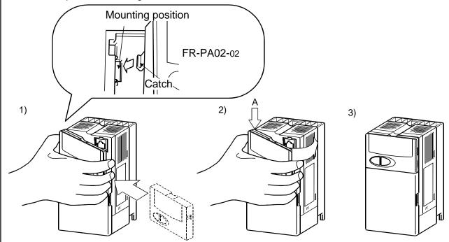
(If the above procedure is not used for removal, the internal connector may be damaged by the force applied.)
