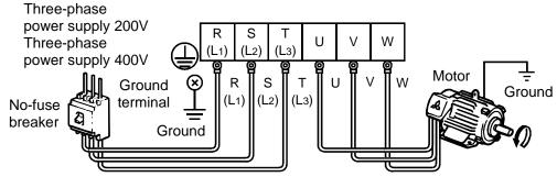
The power supply cables must be connected to R, S, T (L1, L2, L3). If they are connected to U, V, W, the inverter will be damaged. (Phase sequence need not be matched.)
