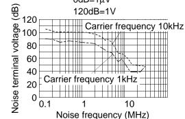
Noise induced to signal cables by inverter output cables
