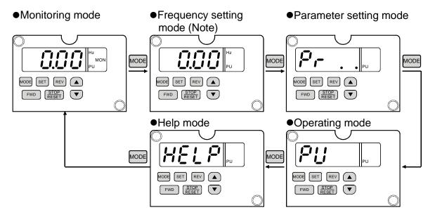
(Note) The frequency setting mode is displayed only in the PU operation mode.
