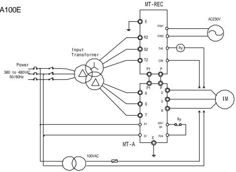
Note : Connect control power supply to terminal R1,S1 on inverter unit
