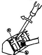
Insert the flat-blade screwdriver into the upper hole ①, and insert the power supply wire into ② while pressing the screwdriver in the direction of the arrow. Remove the screwdriver when the wire has been inserted.
