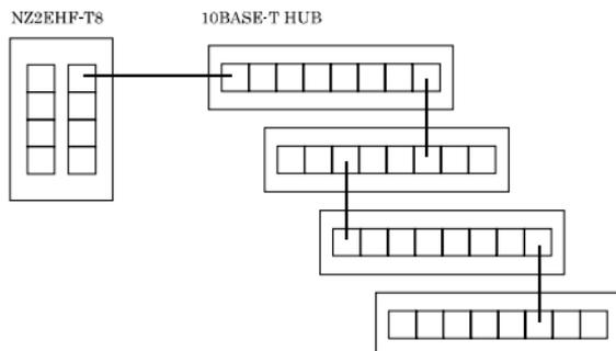
Figure 4.3. Connection restrictions for 10BASE-T repeater HUBs
