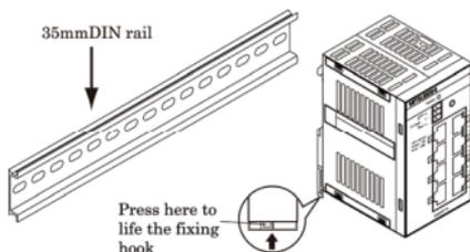
Figure 3.1. Mounting a unit on a DIN rail < 1 / 3 >
