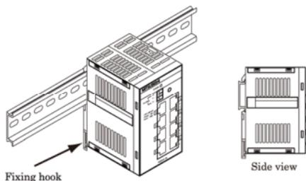
Figure 3.1. Mounting a unit on a DIN rail < 3 / 3 >
