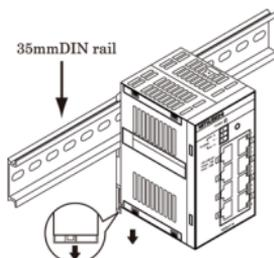
Figure 3.2. Removing a unit from a DIN rail < 1 / 3 >
