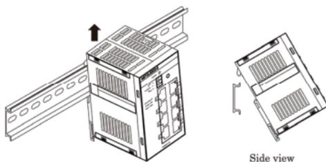
Figure 3.2. Removing a unit from a DIN rail < 3 / 3 >
