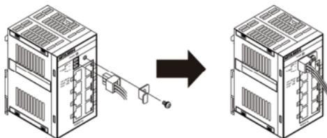
**Figure 3.3. Attaching a retention bracket**
