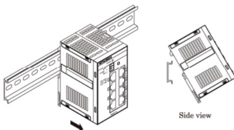
Figure 3.2. Removing a unit from a DIN rail < 2 / 3 >
