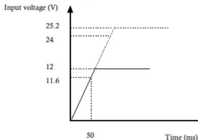
**Figure 2.2. Time required to establish certain voltage**
