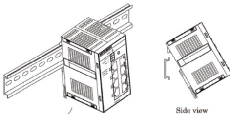
Figure 3.1. Mounting a unit on a DIN rail < 2 / 3 >
