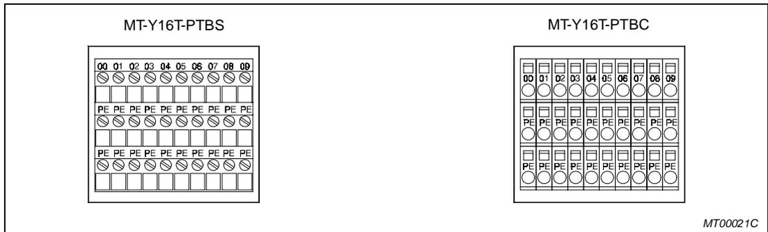
**Fig. 4-17:** Potential terminal blocks MT-Y16T-PTBS and MT-Y16T-PTBC
