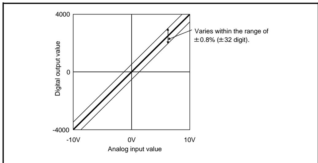
Fig. 3.3 Accuracy of ST1AD2-V
