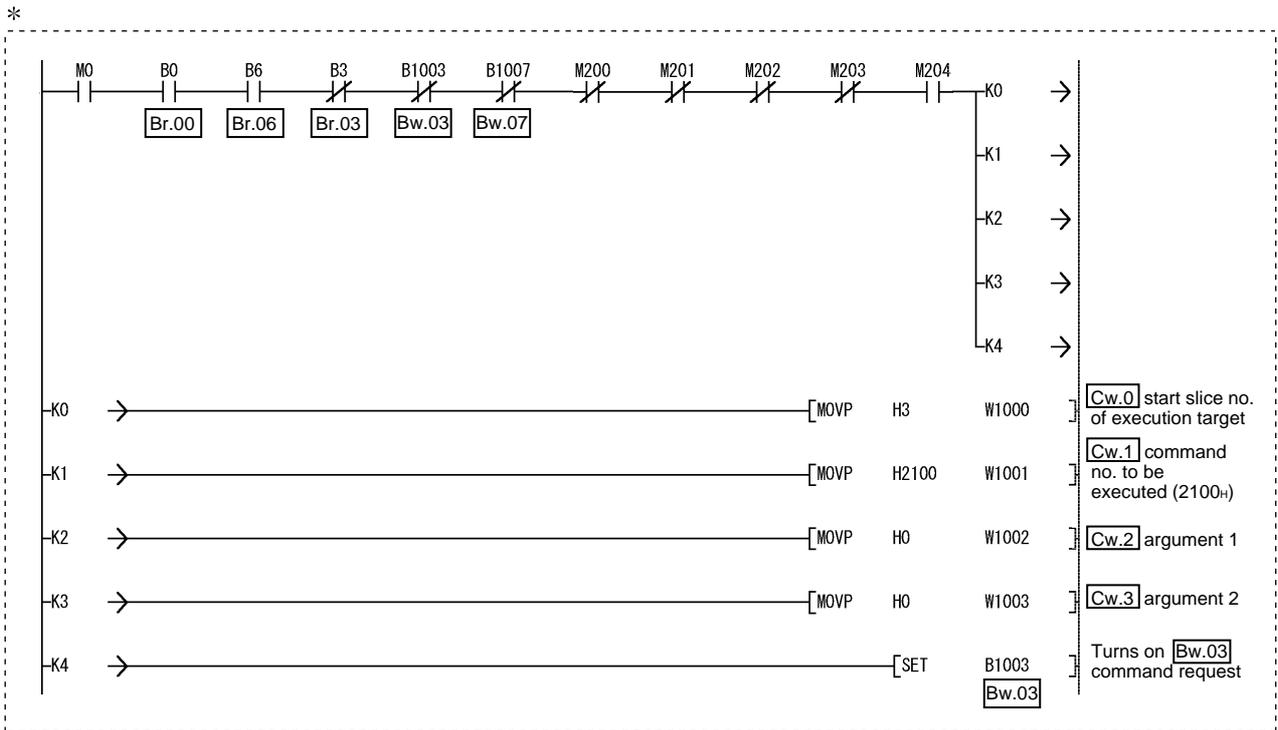
\* The program area enclosed by the dotted line is not required when GX Configurator-ST is used to set the command parameters.
