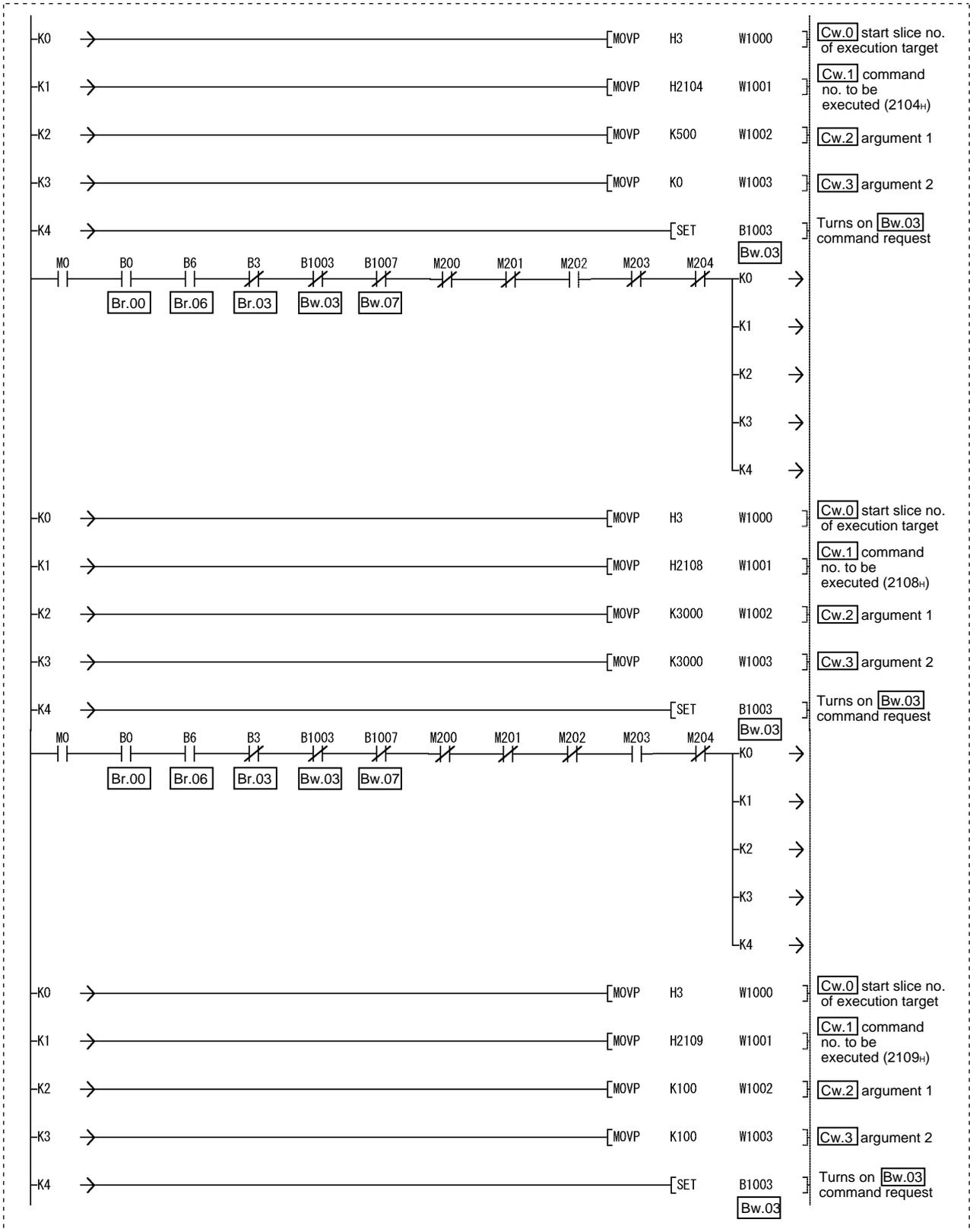
\* The program area enclosed by the dotted line is not required when GX Configurator-ST is used to set the command parameters.
