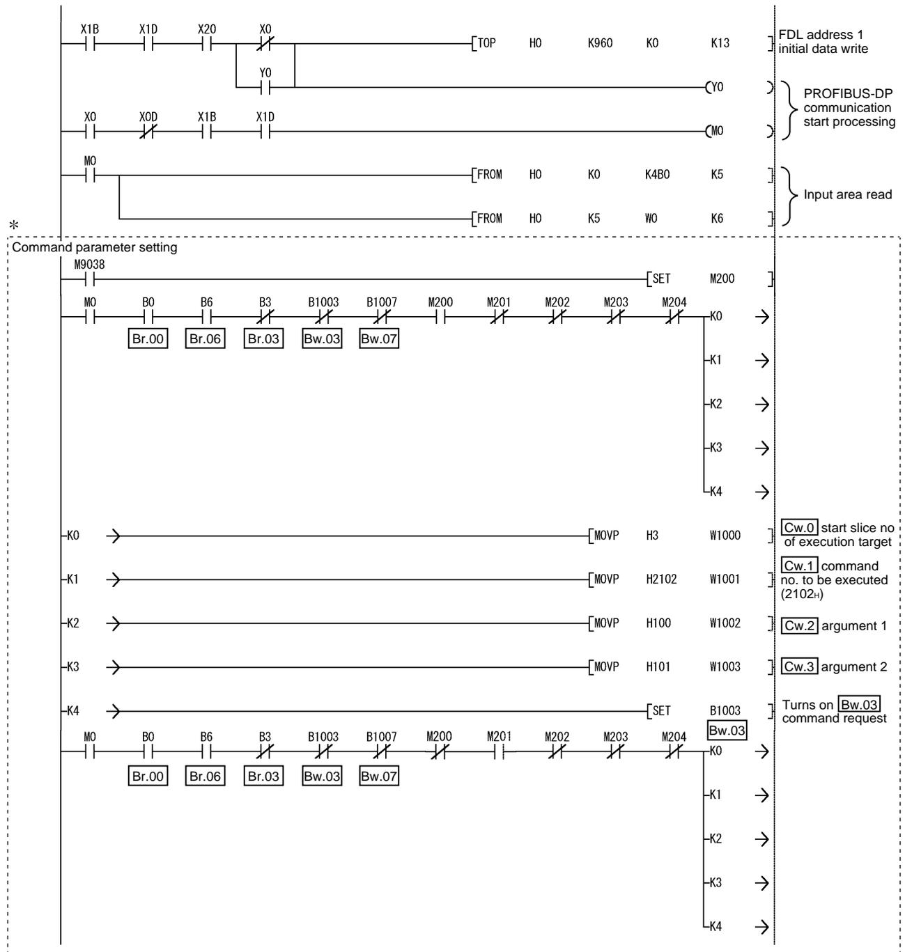
\* The program area enclosed by the dotted line is not required when GX Configurator-ST is used to set the command parameters.
