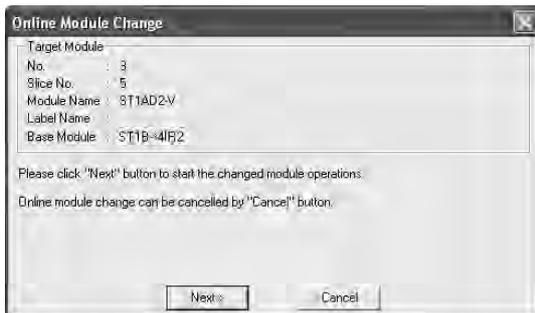
11) After parameter setting or offset/gain setting, execute the operations in steps 1), 2) to resume the online module change.
