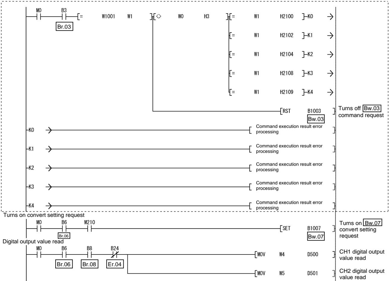
\* The program area enclosed by the dotted line is not required when GX Configurator-ST is used to set the command parameters.
