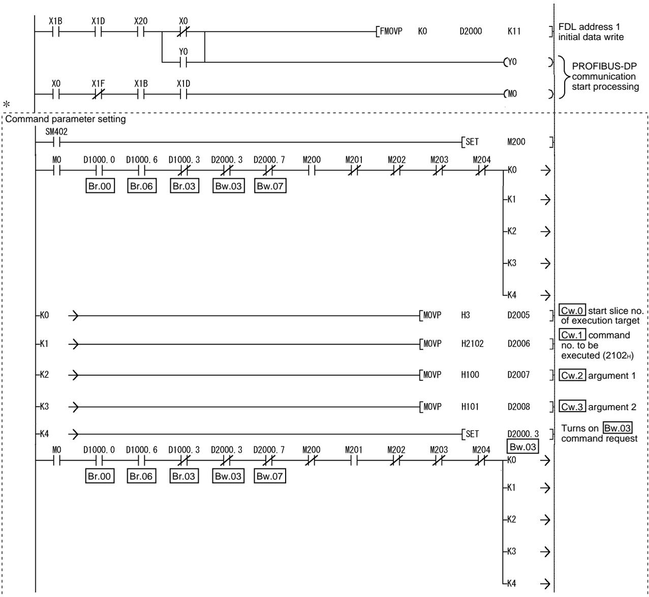
\* The program area enclosed by the dotted line is not required when GX Configurator-ST is used to set the command parameters.
