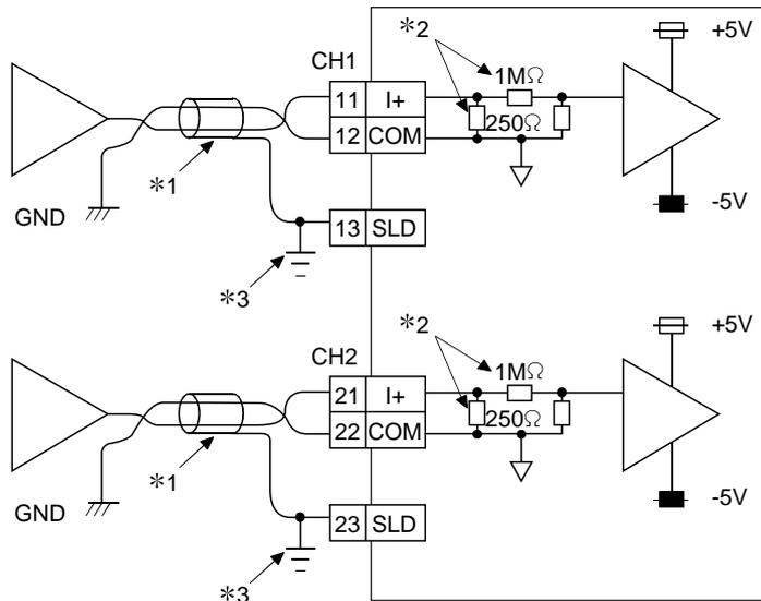
\*1 Use a twisted two core shielded wire for the power wire.
