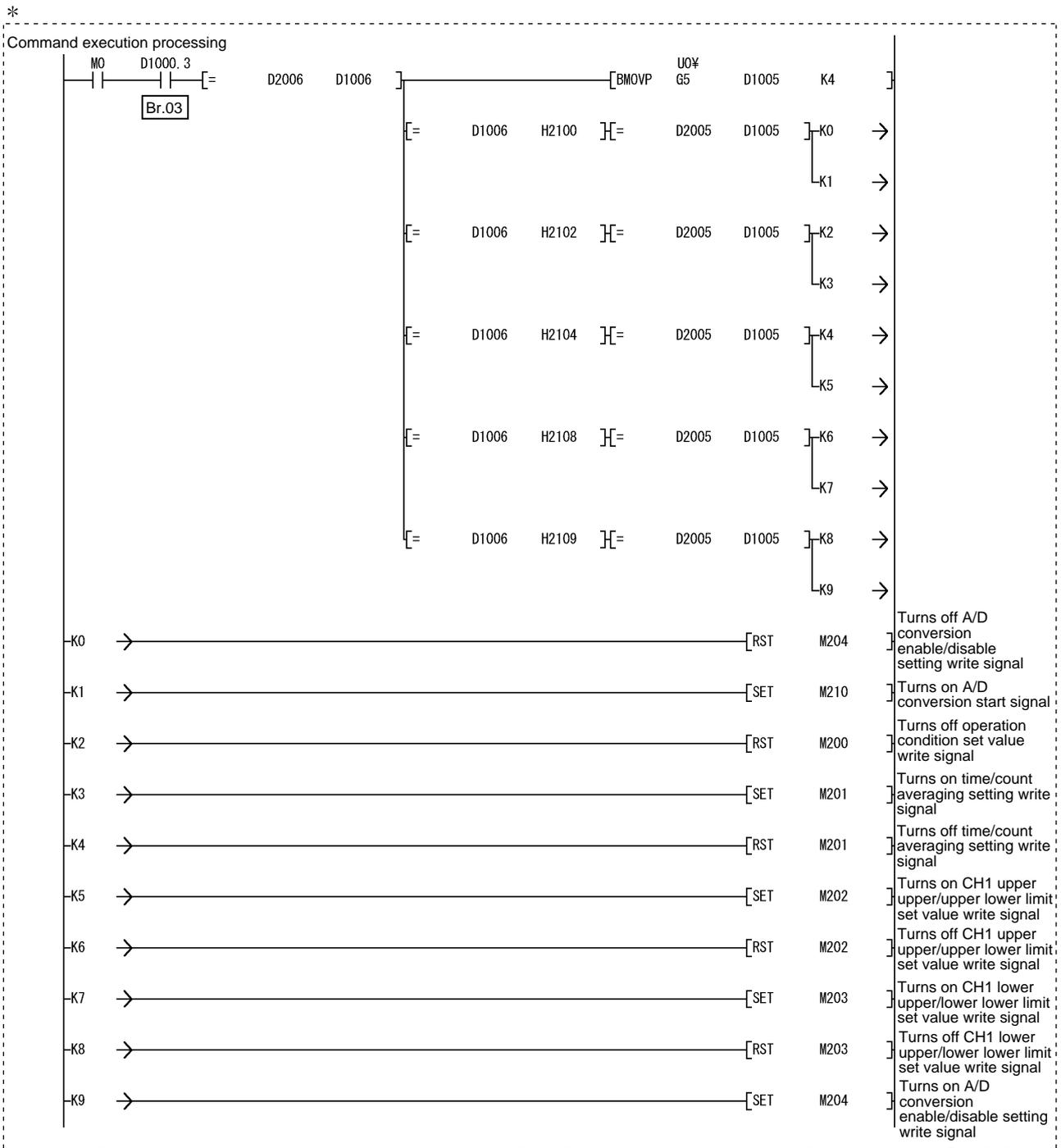
\* The program area enclosed by the dotted line is not required when GX Configurator-ST is used to set the command parameters.
