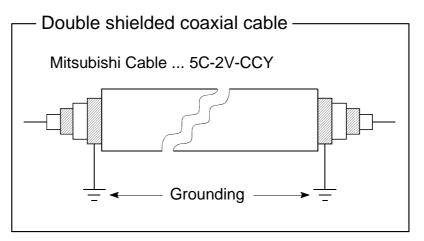
The 5C-2V connector plug is applicable to double-shielded coaxial cable.
