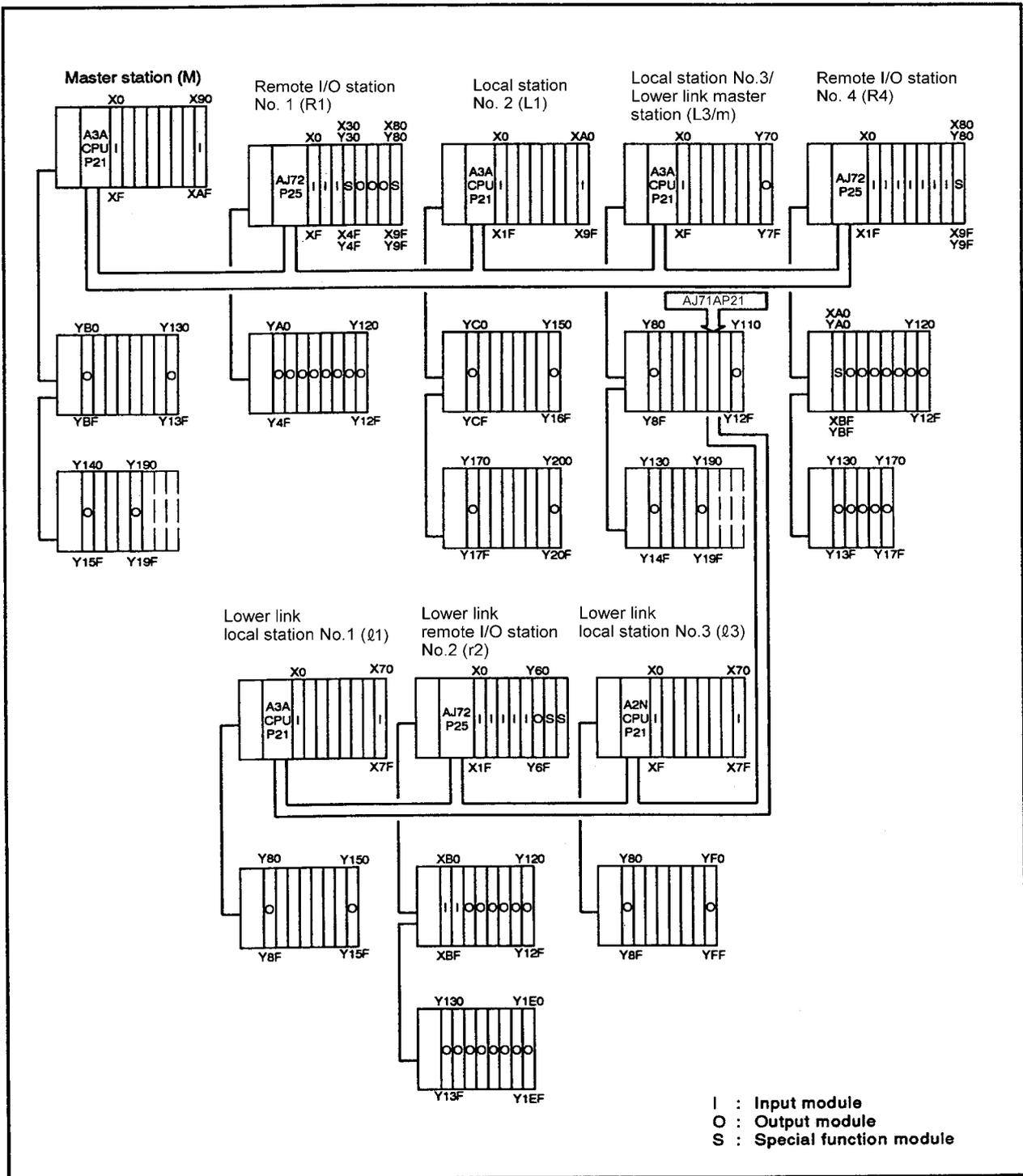
Fig 7.44 Three-tier system configuration example
