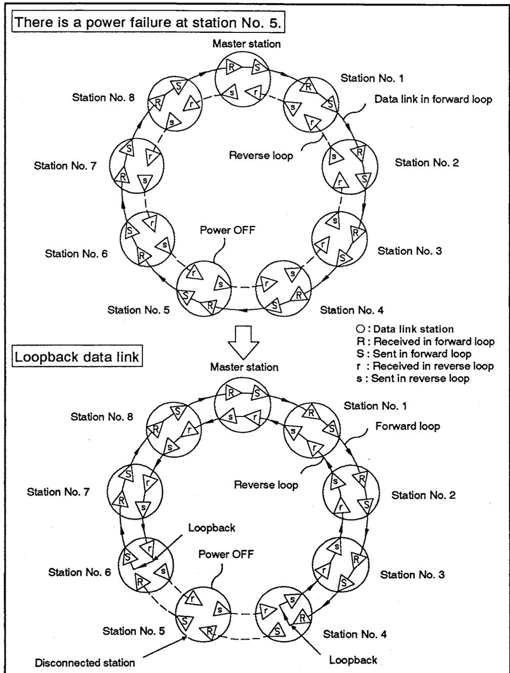
Fig 5.7 Local station or remote I/O station power failure data link
