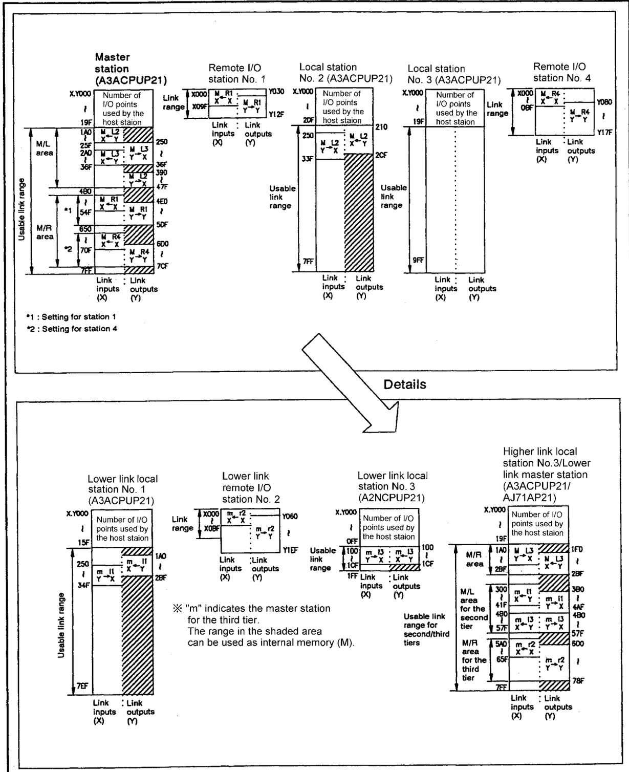
Fig 7.47 Inputs/outputs assignment example
