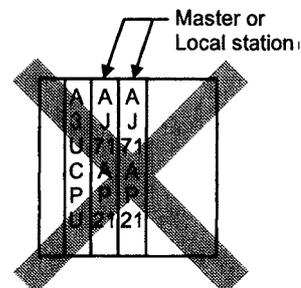
(3) When using a CPU module with link function as a master station for the third tier
