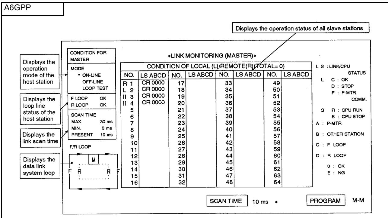
Fig 10.1 Master station link monitor screen (when connecting to master station)
