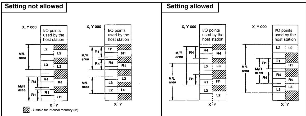
Fig 7.7 Input (X) and output (Y) assignment range
