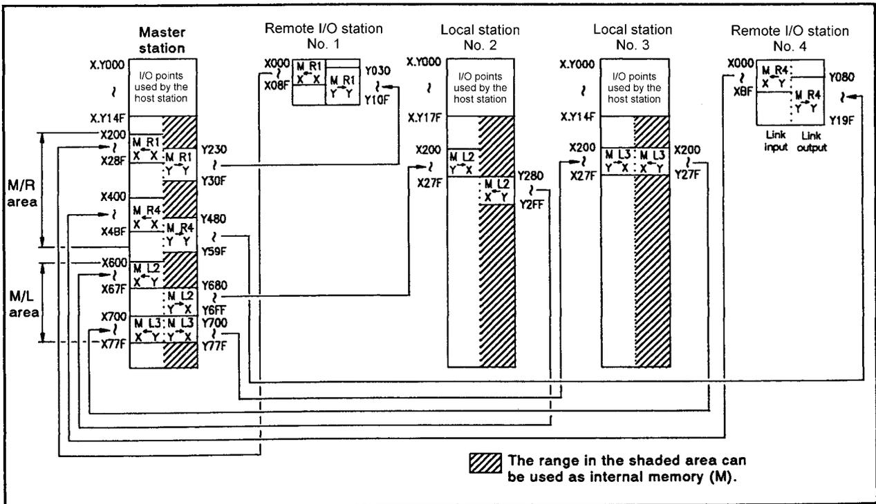
Fig 7.19 Input (X) and output (Y) assignment example
