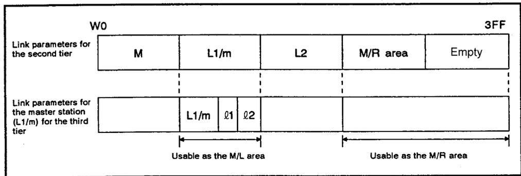
Fig 7.35 Assignment when the MELSECNET mode is used for the third tier
