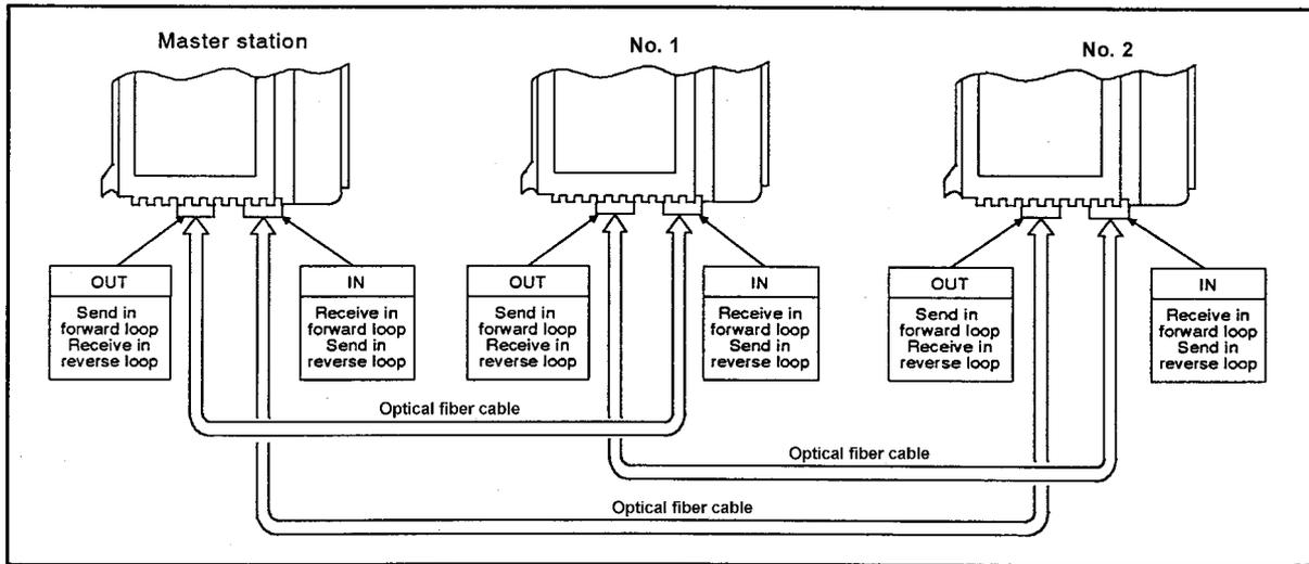
Fig 8.6 Connecting link modules with optical fiber cables
