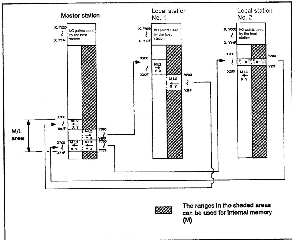
Fig 7.11 Inputs (X) and outputs (Y) assignment example
