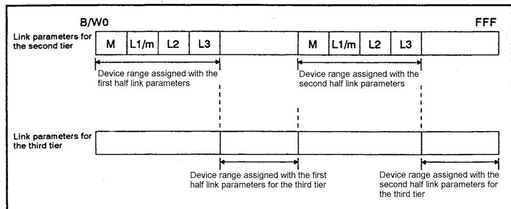
Fig 7.34 Assignment when link relay (B) and link register (W) range is extended
