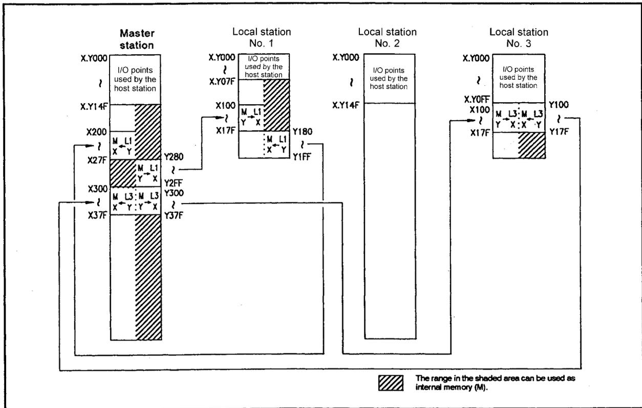
Fig 7.23 Input (X) and output (Y) assignment example
