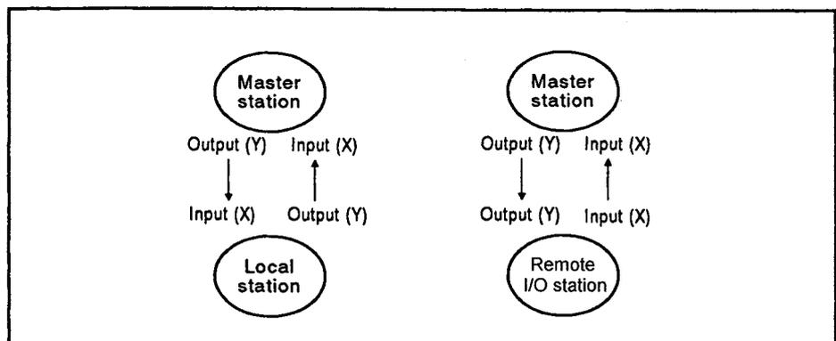
Fig 3.2 Flow of input (X) and output (Y) communication data
