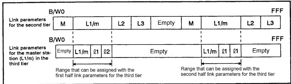
Fig 7.32 When both first and second half link parameters are assigned for second tier
