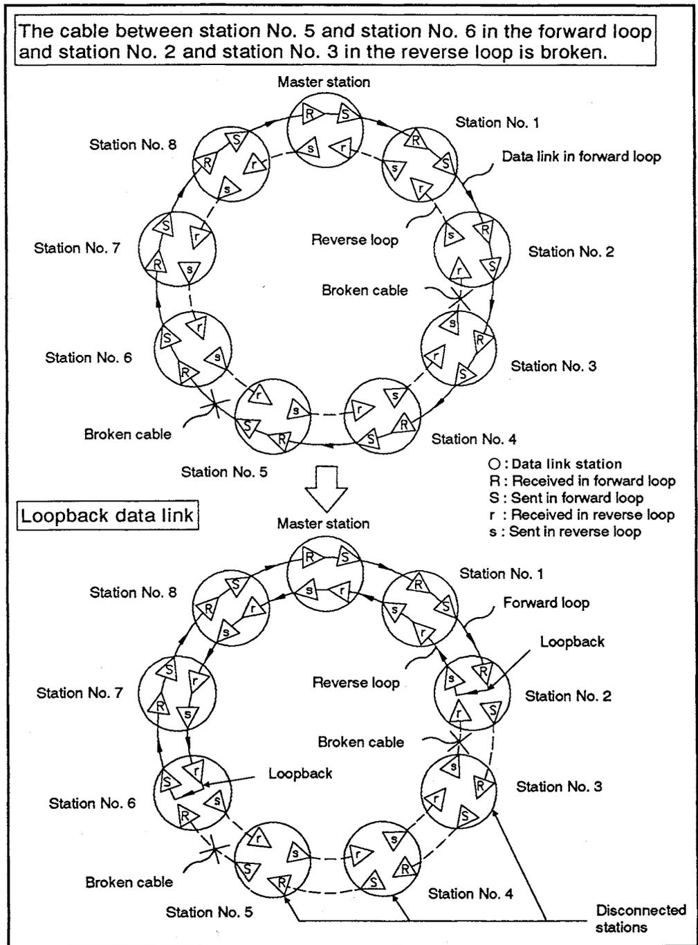
Fig 5.6 Data link when forward/reverse loop is faulty
