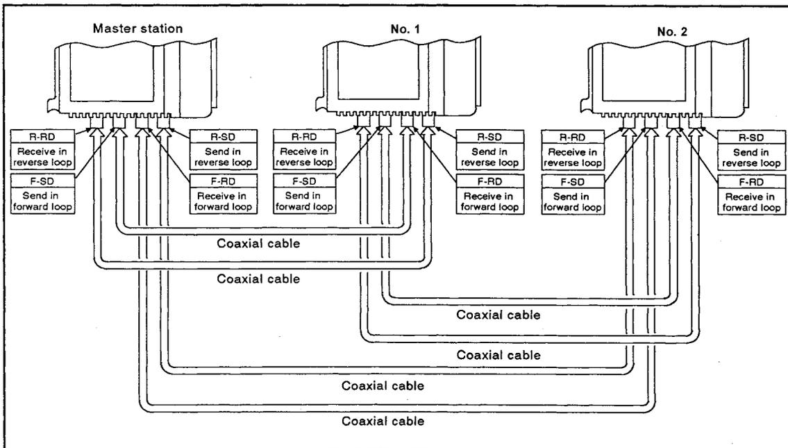
Fig 8.9 Connecting link modules with coaxial cables
