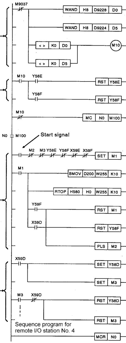
Detects an error in remote I/O station No.4 (when b3 of D9228 is "1").
