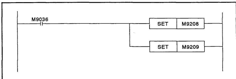
(2) Expanded link relay (B) and link register (W) range
