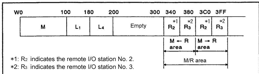
Fig 7.25 Link register (W) assignment example
