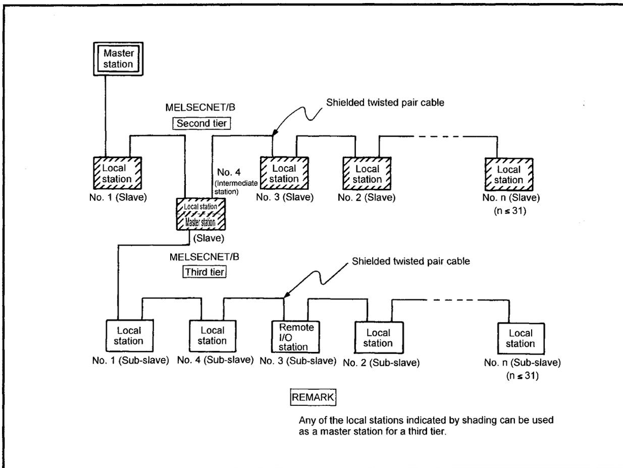
Fig 4.5 Three-tier system configured with MELSECNET/B data link system
