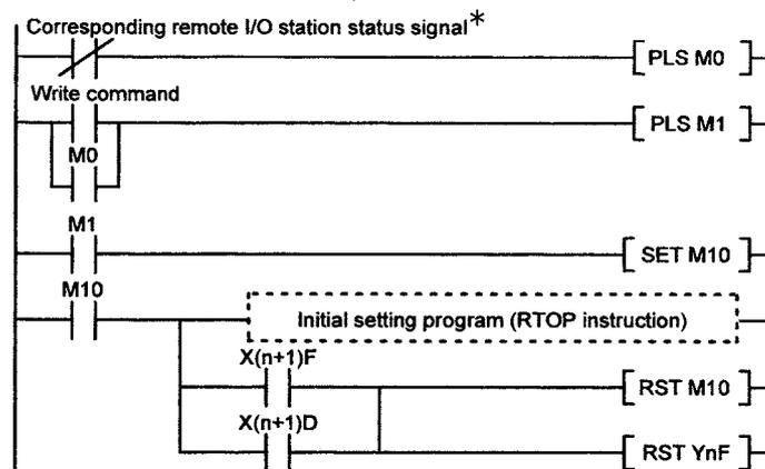
\*: The operating status of the remote I/O station can be checked using remote I/O station error (D9228 to D9231) of special link registers. To use the remote I/O station error in a program, develop it in bit devices M, L, etc. using the MOV instruction. (Example: [MOV D9228 K4M1000], and the contents of D9228 are developed in M1000 to M1015.)
