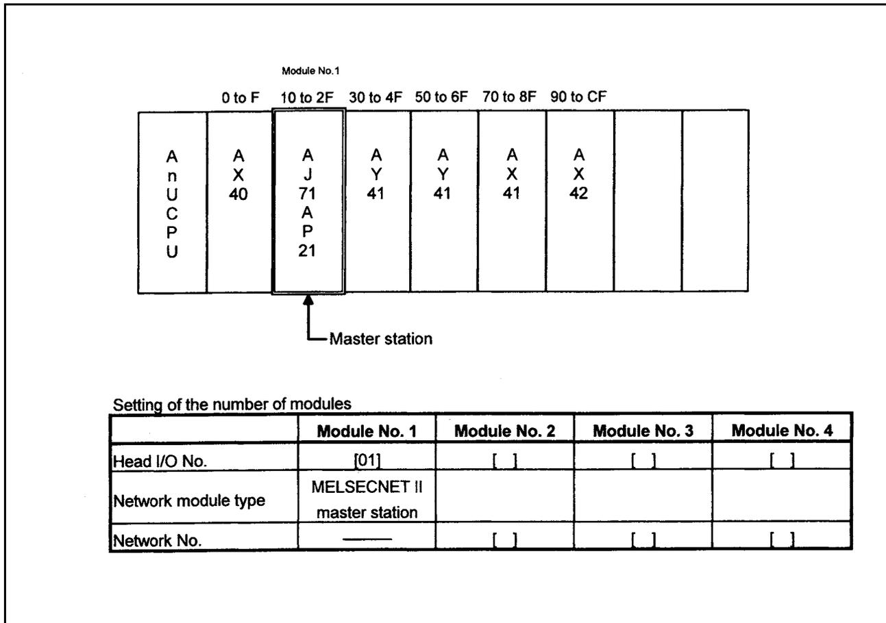
Fig 7.4 System configuration example
