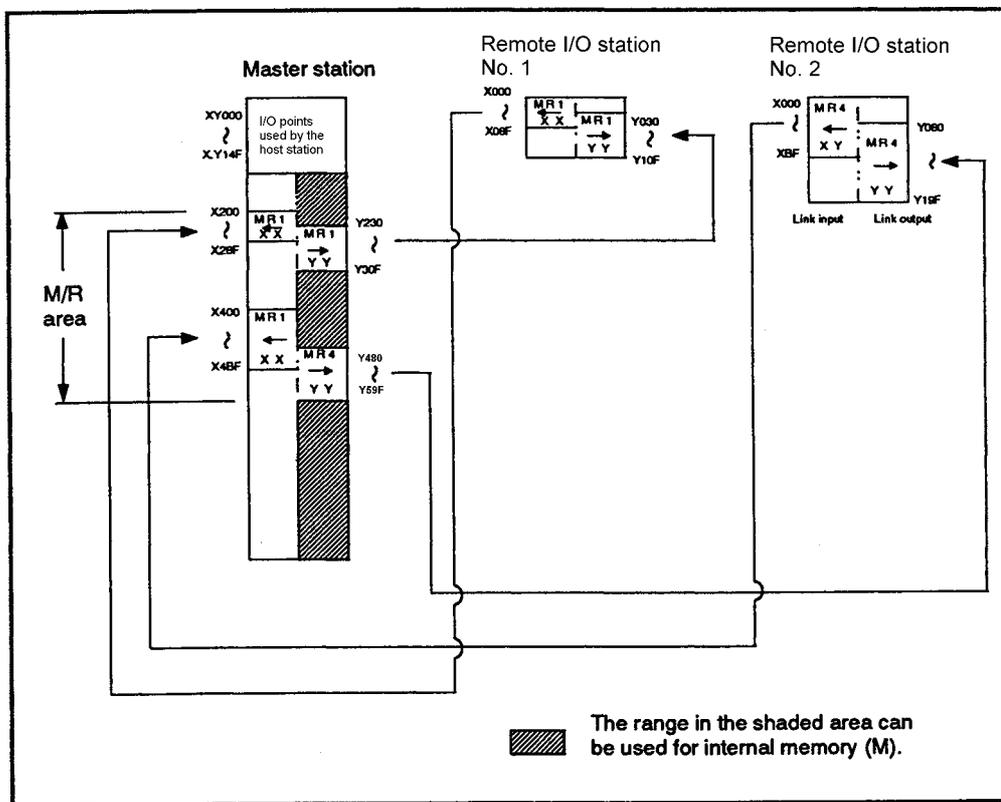
Fig 7.14 Inputs (X) and outputs (Y) assignment example
