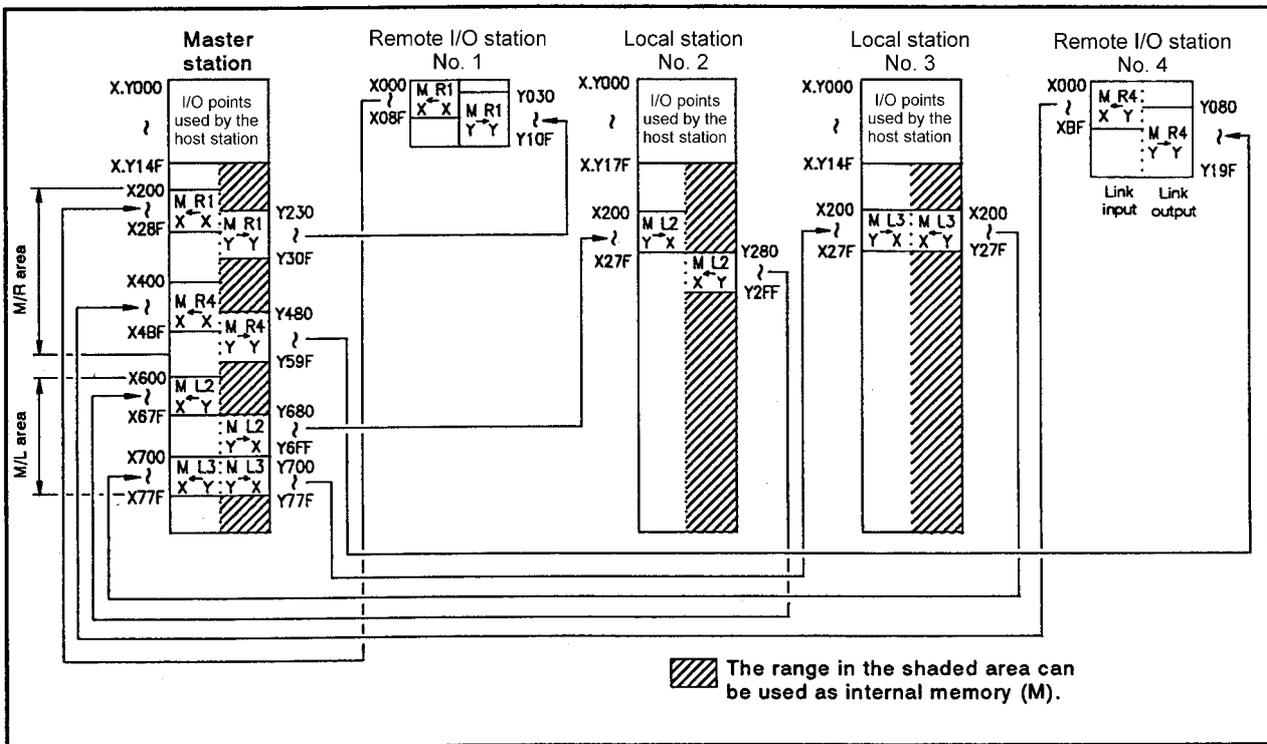
Fig 7.29 Input (X) and output (Y) assignment example
