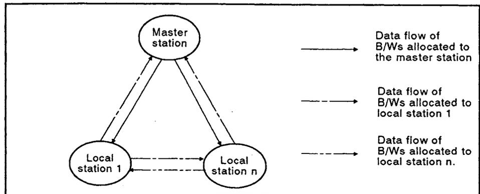
Fig 3.1 Flow of data by B/W communication
