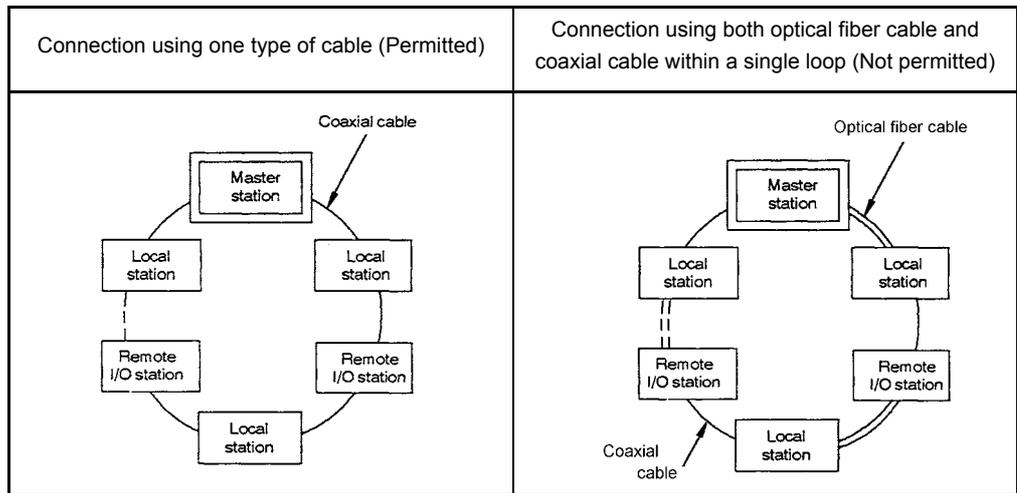
Fig 2.4 Possibility of connection between link modules
