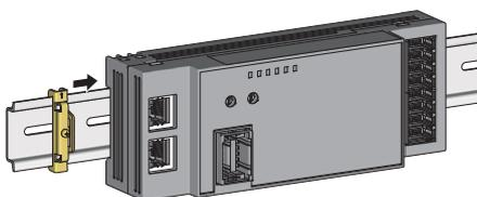
1. Hang the upper latch of the module on the top of the DIN rail.
