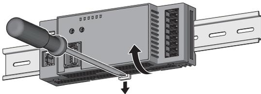
1. Remove the DIN rail stopper. Remove the stoppers from the DIN rail in a procedure opposite to the installation procedure.
