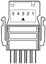
6. Check that there is no gap between the plug body and the plug cover when seen from above. If the latches are not applied properly, a gap appears between the plug body and the plug cover as shown in the incorrect example. To perform crimping as shown in the correct crimping example, be sure to push the plug cover in place with a special tool for crimping.
