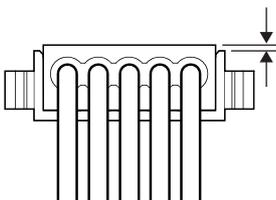
1. Check that the plug cover is attached to the plug body. Do not push the plug cover into the plug body before inserting cables. Once a plug is crimped, it cannot be reused.
