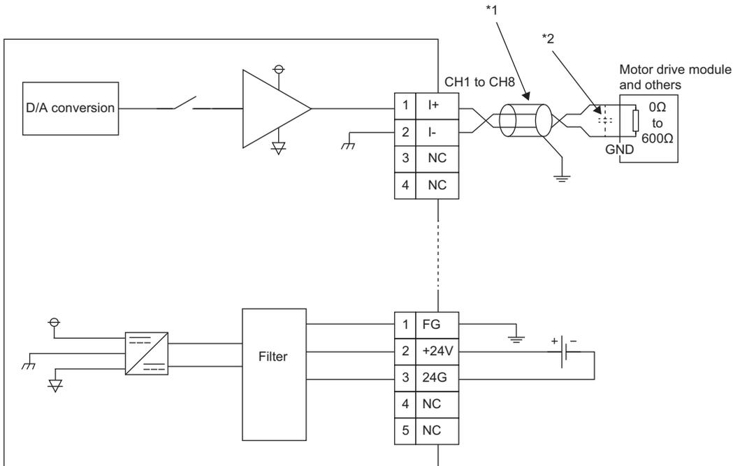
\*1 For the cable, use the 2-core shielded twisted pair cable.
