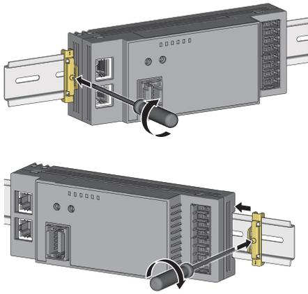
7. Hold the DIN rail stopper in the direction opposite to the arrow on the stopper and tighten the screw with a screwdriver.
