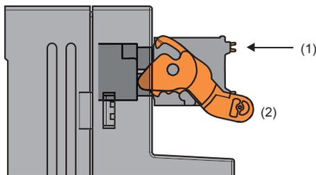
Figure viewed from the module top surface: When insertion of the terminal block has completed
