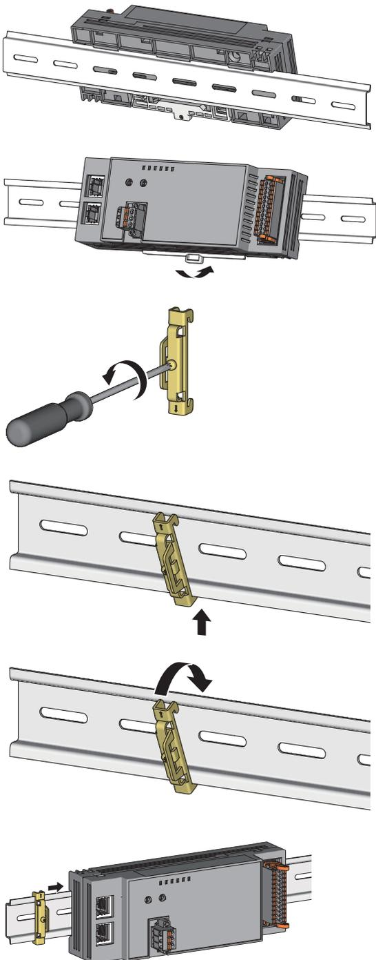
1. Hang the upper tabs of the module on a DIN rail.
