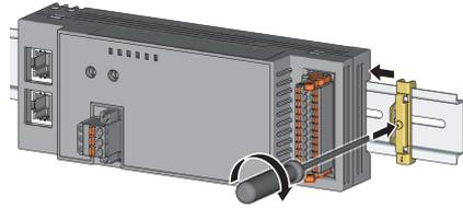
8. Install the DIN rail stopper on the right side of the module in the same procedure.
