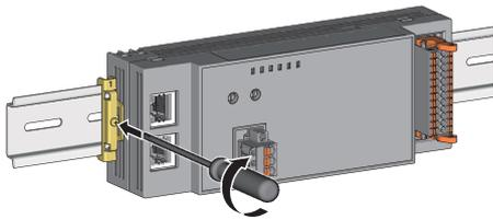
7. Hold the DIN rail stopper in the direction opposite to the arrow on the stopper and tighten the screw with a driver.
