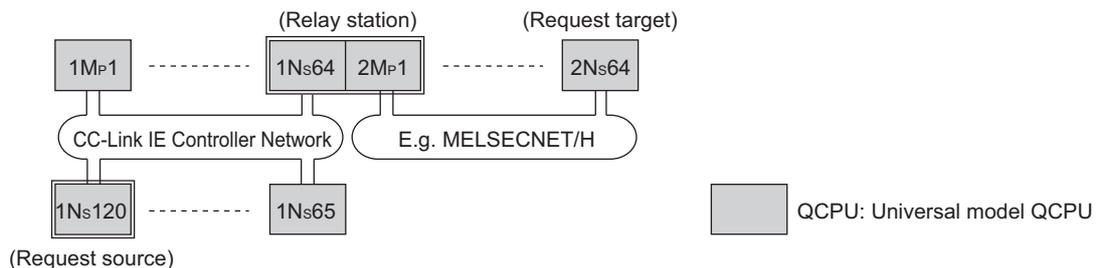
2) When the relay station number of the CC-Link IE Controller Network is 65 or higher
