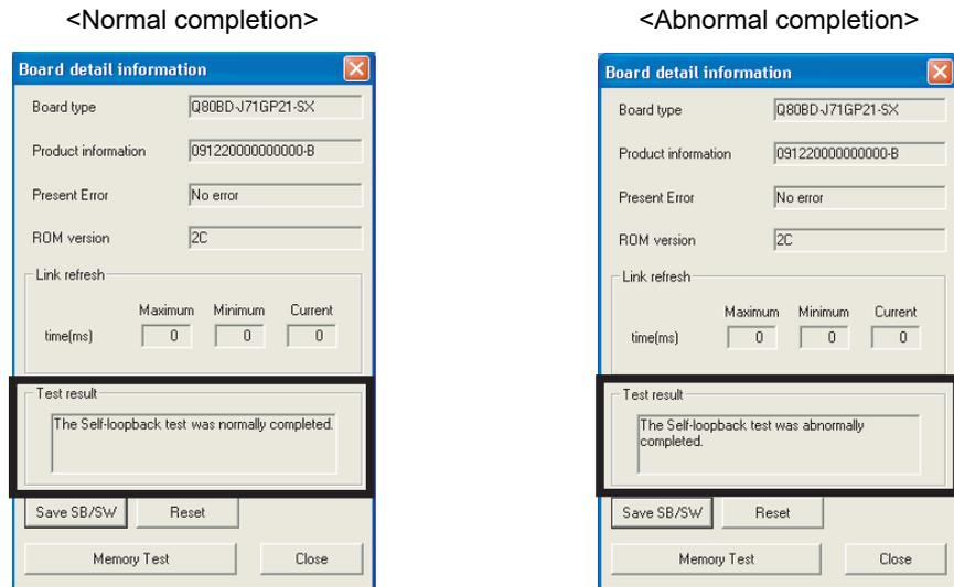
If the test completes abnormally, replace the optical fiber cable and execute the test again.
