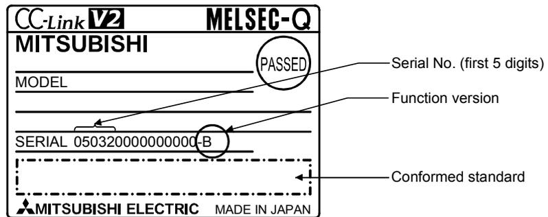
(When checking the function version on GX Developer)
