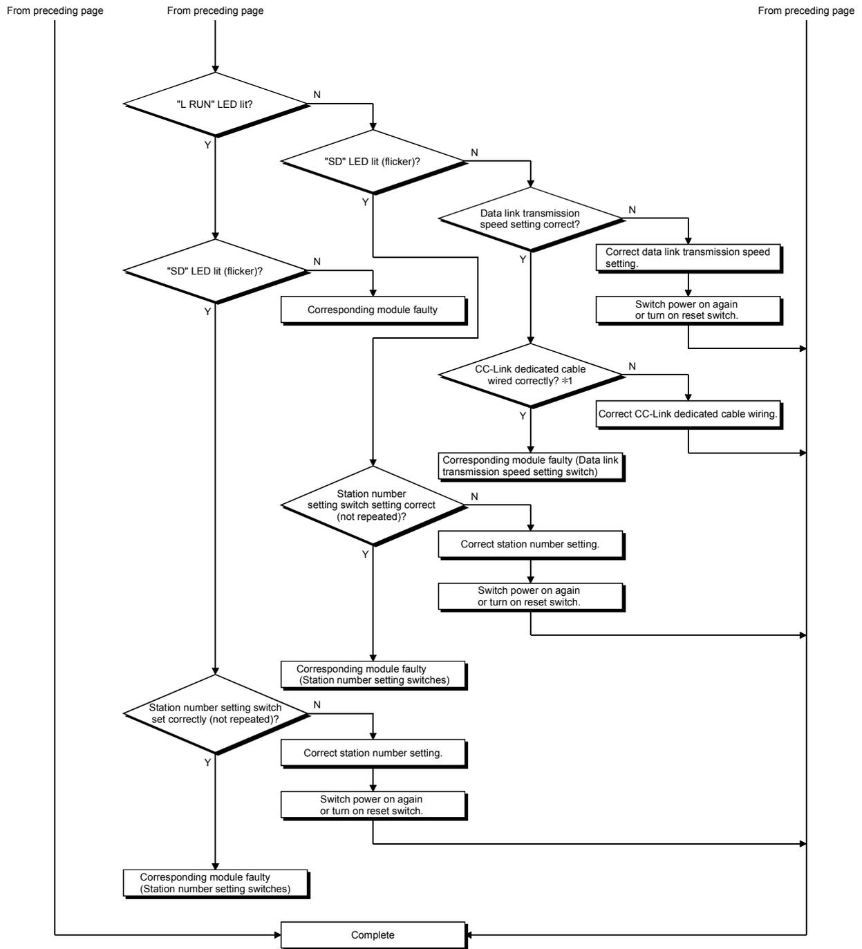
\*1: Check for short circuit, reverse connection, wire breakage, no terminal resistor, improper FG connection, improper overall distance and improper interstation distance.
