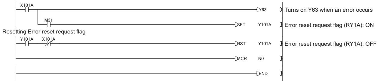
Figure 5.8 Program example (when using the QCPU (Q mode)) 2/2
