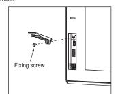
To use the USB interface, open the USB environmental protection cover by pushing the [PUSH] mark on the cover.
