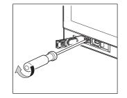
4) When you do not use the USB interface, close the USB environmental protection cover by pushing in the [USB] mark on the cover firmly. When you close the USB environmental protection cover, make sure that the latch is fully retracted into the cover body. Otherwise, the USB environmental protection cover may get damaged.
