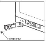
5) To use the USB interface, unlock the USB environmental protection cover by sliding its latch and then open the cover.
