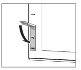
Tighten the fixing screw in the specified torque range (0.36 N•m to 0.48 N•m) to fix the cover to the GOT.
