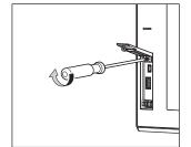
4) When you do not use the USB interface, close the USB environmer protection cover by pushing in the [PUSH] mark on the cover firmly.
