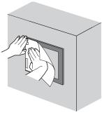
3) To attach the protective sheet, attach it from one direction gradually. Make sure to fit the protective sheet onto the joining surface closely without leaving any air
