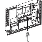
8) Insert two cable ties into the cable tie mount, and secure the HDMI cable by
