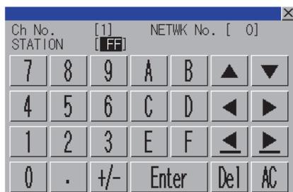
4. After selecting the station number, touch the enter key. The communication setting window closes and the system configuration of the set monitor destination is displayed.
