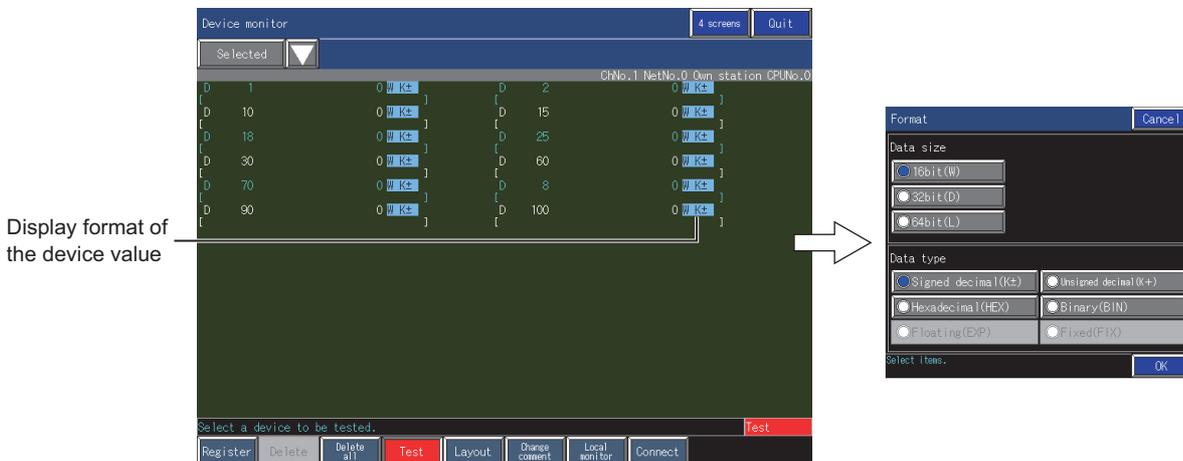
**4.** Touch a device targeted to the test operation.
