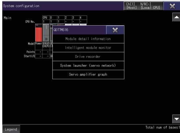
4. Touch the system launcher (servo network) from the function list to display the servo network configuration diagram.
