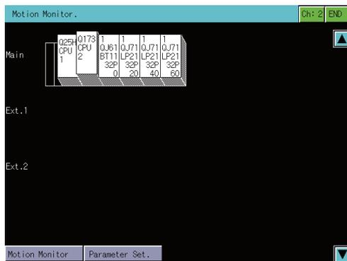
5. Touch the [Parameter Set.] key to display the parameter setting screen.
