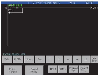
After searching for coil M120 that is in the OFF state, "M669" and "M23" are displayed as devices that are not conductive.
