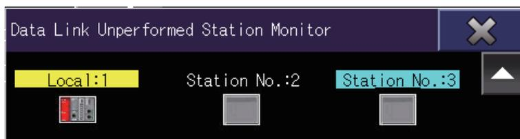
During the CC-Link IE Field Network diagnostics, when the master station has the serial number starting with 17021 or earlier in the first 5 digits, updating the network configuration diagram deletes the disconnected stations.
