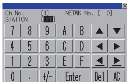
3. After selecting the station number, touch the [Enter] key. The communication setting window closes and the system configuration of the set monitor destination is displayed.
