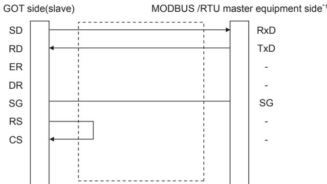
\*1 Some MODBUS/RTU master equipment require the control line (CS, RS, etc.) to be controlled. Make sure to connect the cables and wires as described in the MODBUS/RTU master equipment manual.
