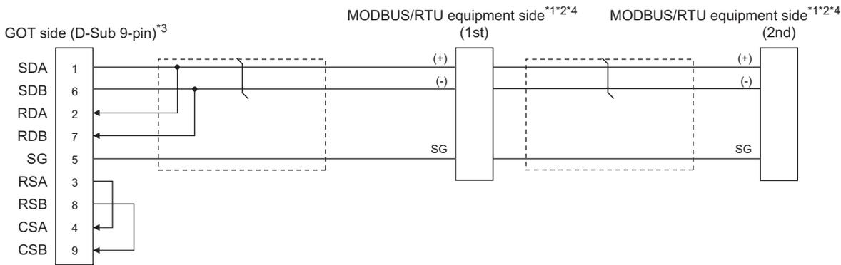
\*1 The actual terminal layout on the MODBUS/RTU equipment may differ from the example shown above. SDA/B(+/-) and RDA/B(+/-) terminals can be separated from each other. Make sure to connect the cables and wires as described in the MODBUS/RTU equipment manual.
