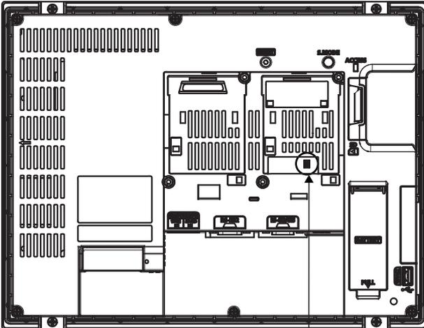
Terminating resistor setting switch
