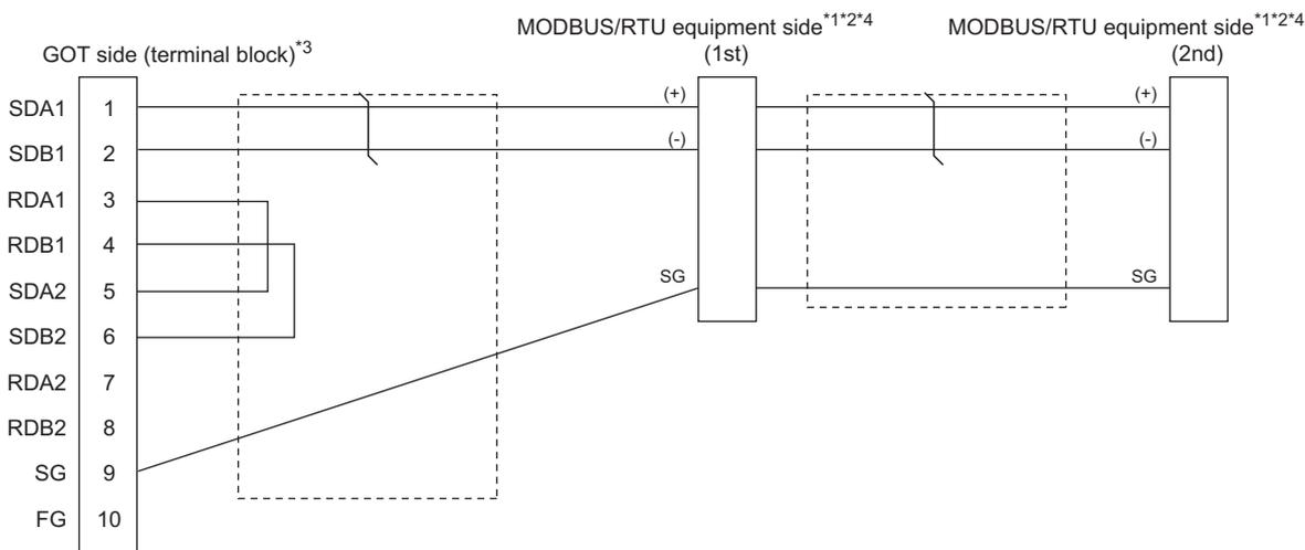
\*1 The actual terminal layout on the MODBUS/RTU equipment may differ from the example shown above. SDA/B(+/-) and RDA/B(+/-) terminals can be separated from each other. Make sure to connect the cables and wires as described in the MODBUS/RTU equipment manual.
