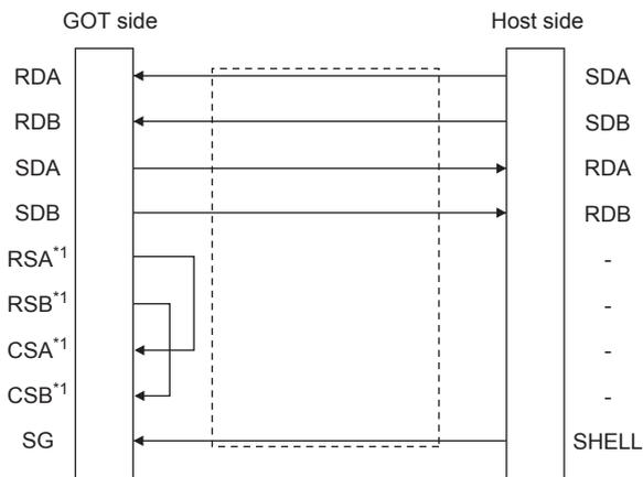
\*1 The signals RSA, RSB, CSA, and CSB are not provided for GT2104-PMBD, GT2103-PMBD. Return connection is not required.
