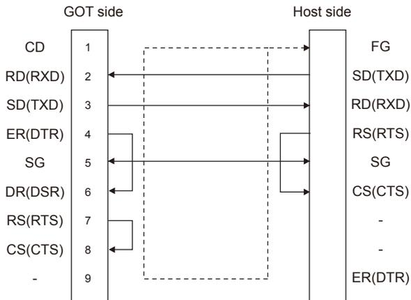
Example of the case where the DTR/DSR signal is used
