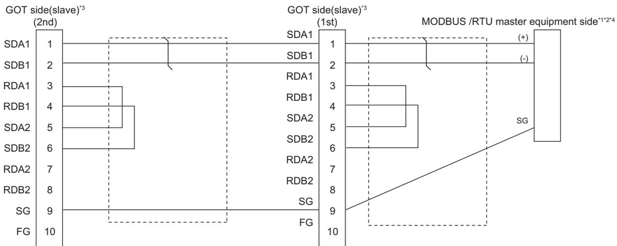
\*1 The actual terminal layout on the MODBUS/RTU master equipment may differ from the example shown above. SDA/B(+/-) and RDA/B(+/-) terminals can be separated from each other. In such cases, make sure to connect the cables and wires as described in the MODBUS/RTU master equipment manual.
