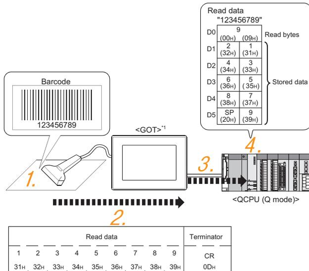
\*1 The GOT and QCPU (Q mode) are connected through a bus.
