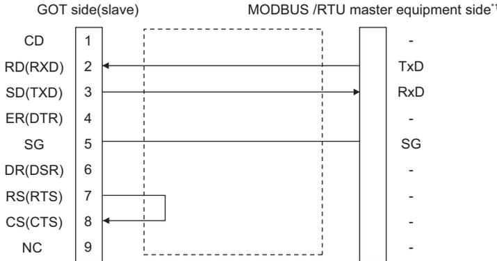
\*1 Some MODBUS/RTU master equipment require the control line (CS, RS, etc.) to be controlled. Make sure to connect the cables and wires as described in the MODBUS/RTU master equipment manual.
