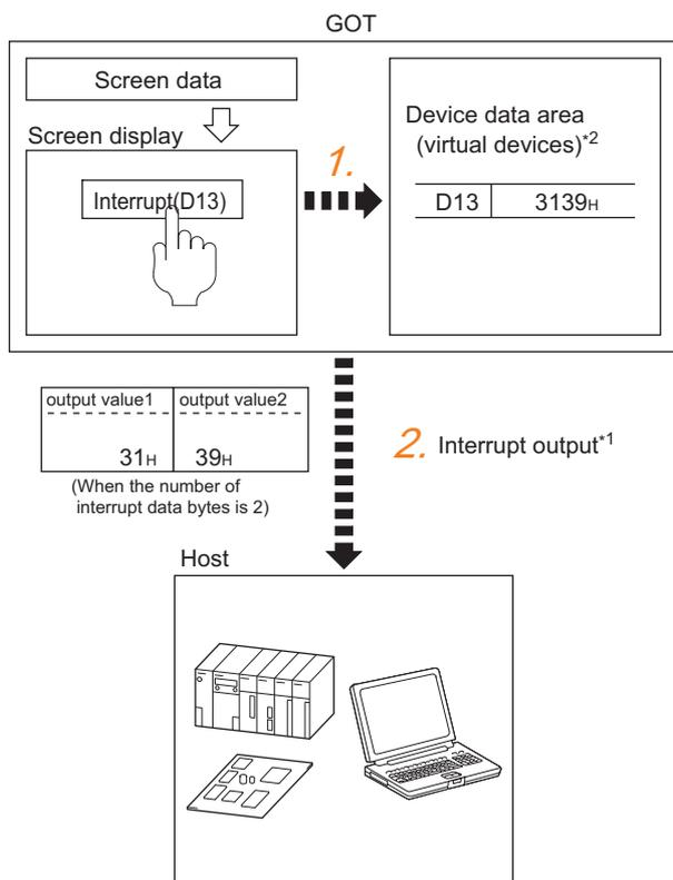
1. Data are written to the virtual devices for interrupt output from the touch switches on the GOT.
