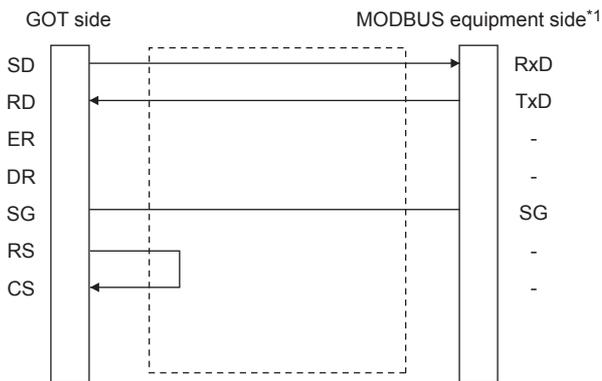
\*1 Some MODBUS/RTU equipment require the control line (CS, RS, etc.) to be controlled. Make sure to connect the cables and wires as described in the MODBUS/RTU equipment manual.
