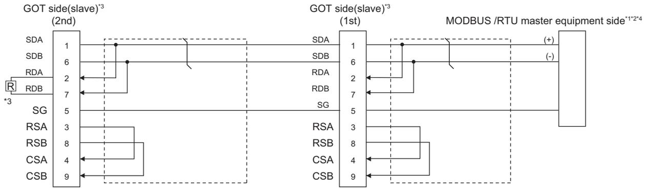
\*1 The actual terminal layout on the MODBUS/RTU master equipment may differ from the example shown above. SDA/B(+/-) and RDA/B(+/-) terminals can be separated from each other. In such cases, make sure to connect the cables and wires as described in the MODBUS/RTU master equipment manual.
