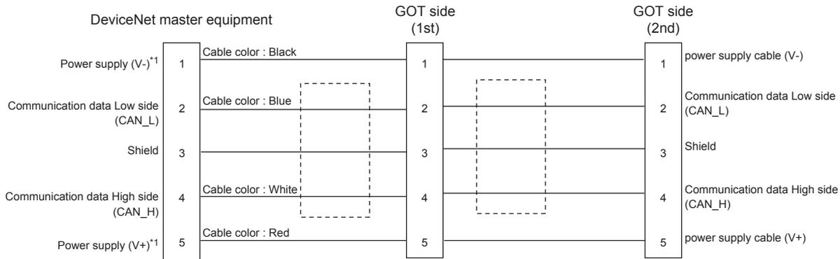
\*1 The power supply for communication (24 V DC) is required to supply the power to the power supply (V-) and power supply (V+).
