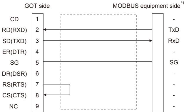
\*1 Some MODBUS/RTU equipment require the control line (CS, RS, etc.) to be controlled. Make sure to connect the cables and wires as described in the MODBUS/RTU equipment manual.
