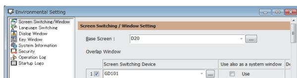
2. Set D20 to the screen switching device (base screen).
