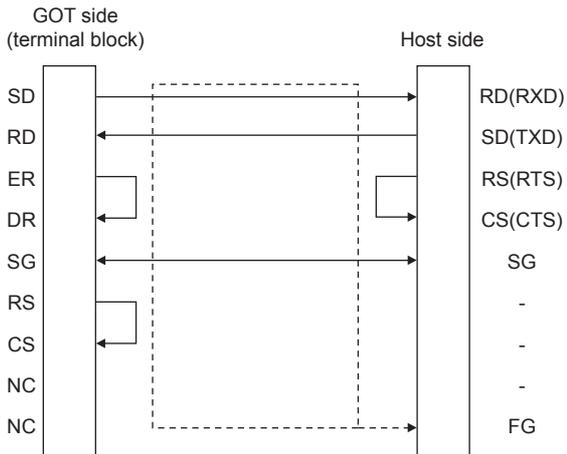
Example of the case where the DTR/DSR signal is used
