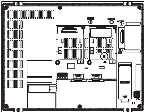
Terminating resistor setting switch
