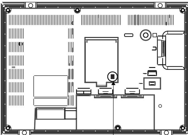
Terminating resistor setting switch
