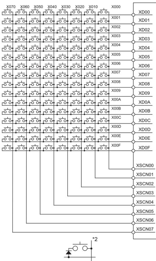
\*1 The 128-point input can be executed with using a 16-point input signal (XD00 to XD0F) with an 8-point scan signal (XSCN00 to XSCN07).
