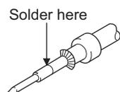
**5.** Insert the contact assembly shown in step 4 into the plug shell and screw the nut into the plug shell.
