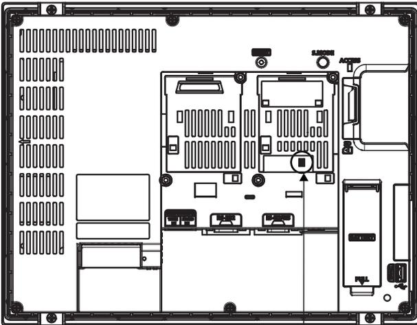
Terminating resistor setting switch
