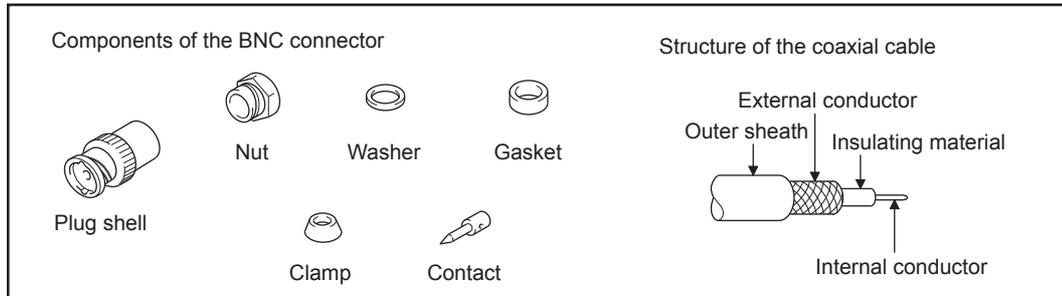
1. Remove the external sheath of the coaxial cable with dimensions as shown below.
