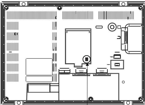
Terminating resistor setting switch
