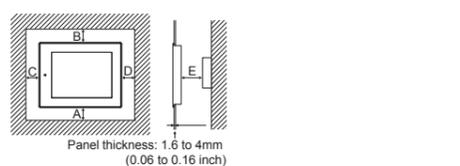
According to the dimensions in the following table, leave clearances between the GOT and the other devices. The values enclosed in square brackets apply to the case where no other equipment generating radiated noise (such as a contactor) or heat is installed near the GOT. However, keep the ambient temperature of the GOT to 55°C or lower.
