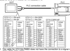
\*1 The cable for GT2104-PMBD does not have the connection to a signal name (RSA, RSB, CSA, CSB).
