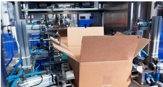
Simple synchronous operations including horizontal, vertical, and rotational movements are possible with a start signal to all axes via cyclic transmission. This function can be used to easily build a multi-axis system for packaging, etc.
