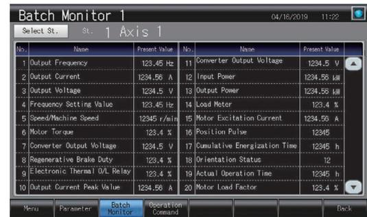
With GOT, the replacement timing of the inverter's components can be displayed and predictive maintenance can be performed!
