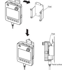
The figure shows an image of attaching the Handy GOT to the wall-hanging
