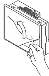
1) If a protective sheet is on the GOT, peel off the protective sheet from the bottom-right corner of the GOT display section, and clean the GOT surface.
