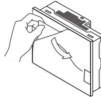
3) Peel off the protective film on the protective sheet.
