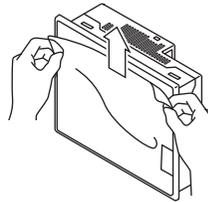
2) Peel the release paper from the back of the new protective sheet, and attach its adhesive side to the GOT display section. When attaching the protective sheet, make sure to fit it on the display section closely without leaving any clearance between them.
