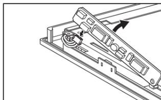
When replacing GT15-80SLTT, remove the cable from the cable holder. (When replacing GT15-80SLTT)
