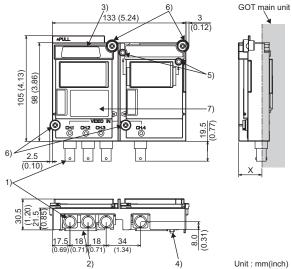
Dimensions of X when the video input unit is mounted to the GOT
