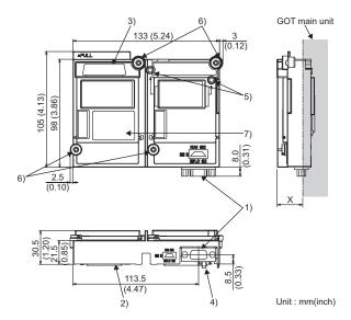
Dimensions of X when the RGB input unit is mounted to the GOT.
