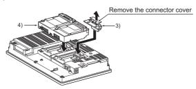
(5) Fasten the MELSECNET/H communication unit by tightening its mounting screws (4 places) with tightening torgue 0.36 to 0.48 N•m. (6) Fasten the bus connection unit by tightening the board fixing screws (2 places) with the tightening torque of 0.36 to 0.48 N•m.
